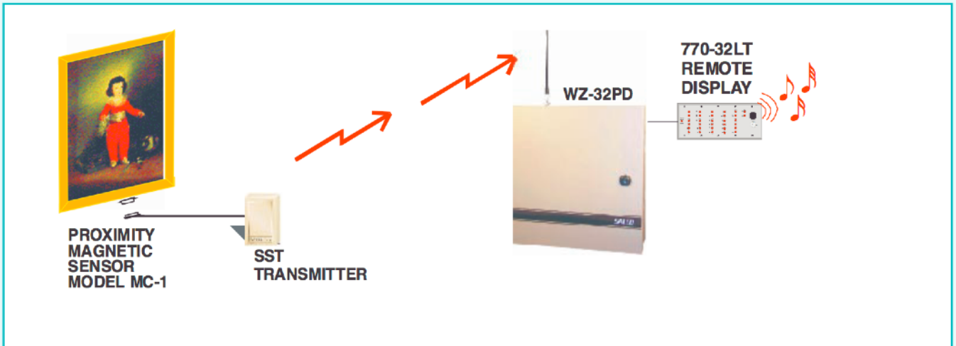
Proximity Magnetic Sensor Installed Behind A Painting
