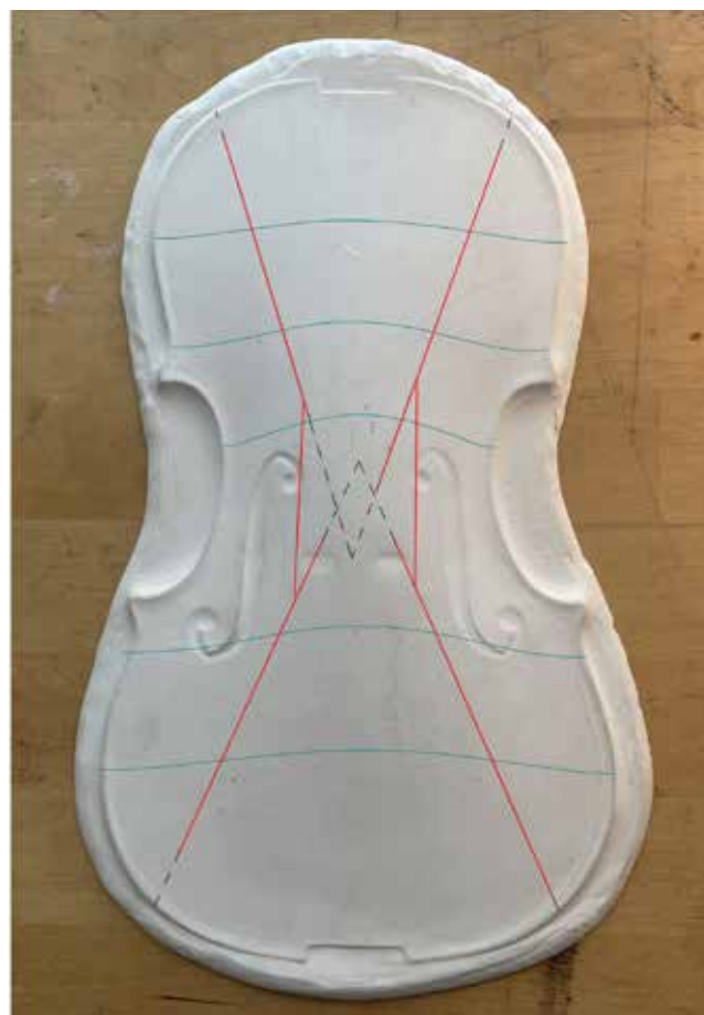
FIGURE 4 Cast of the 'Ole Bull' top, showing the straight lines (red), their extensions (dotted black), and the cross sections (blue)
