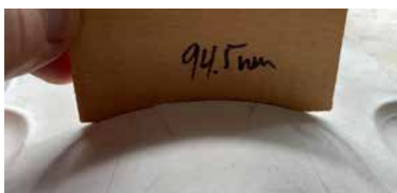
FIGURE 5 The C-bout cross-section of the LAS forms a radius
