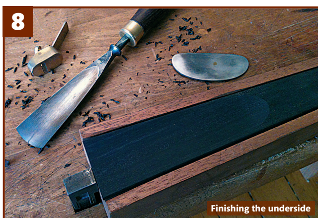
This fingerboard is tapered on the underside
