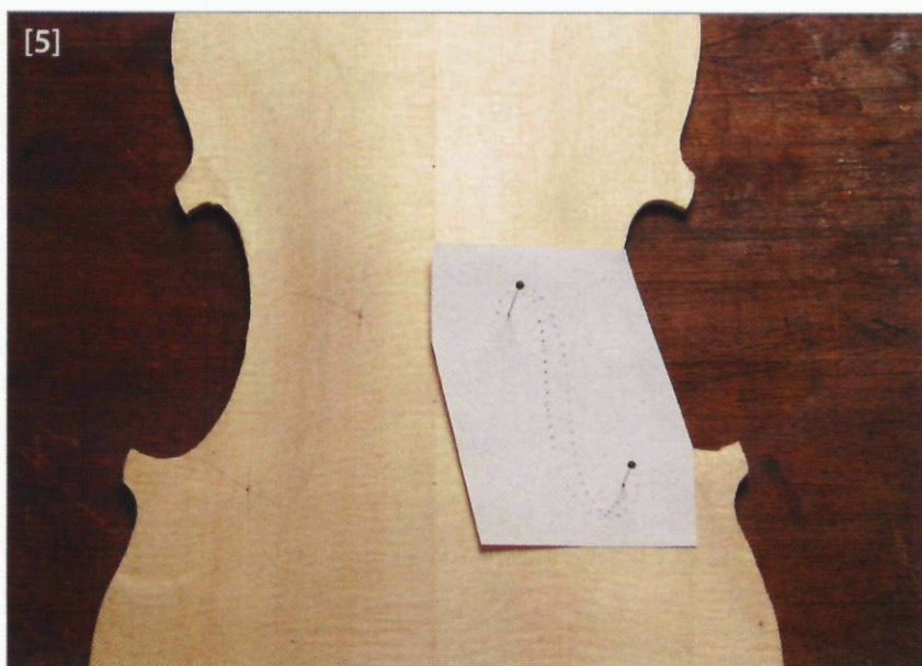
[5] Transferring the f-hole design to the top using a pounce template
