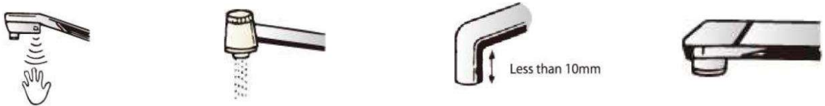
Sensor operated Retractable shower head Shallow faucet Unusual thread diameter
