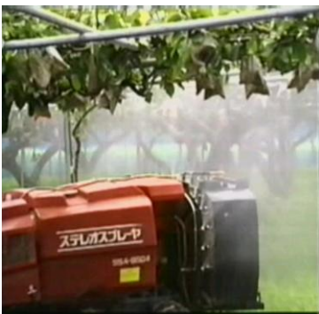
GROWER WITH STANDARD ORCHARD SPRAYER DELIVERING FEW IN MIST FORM
