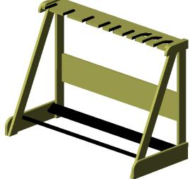
This design has many individual parts and two layers, each in a different colour. In GstarCAD, save the file as a normal AutoCAD 2018 (or whatever version you use).**Dwg** file first then for the conversion, save it as an AutoCAD r12 .DXF file.
