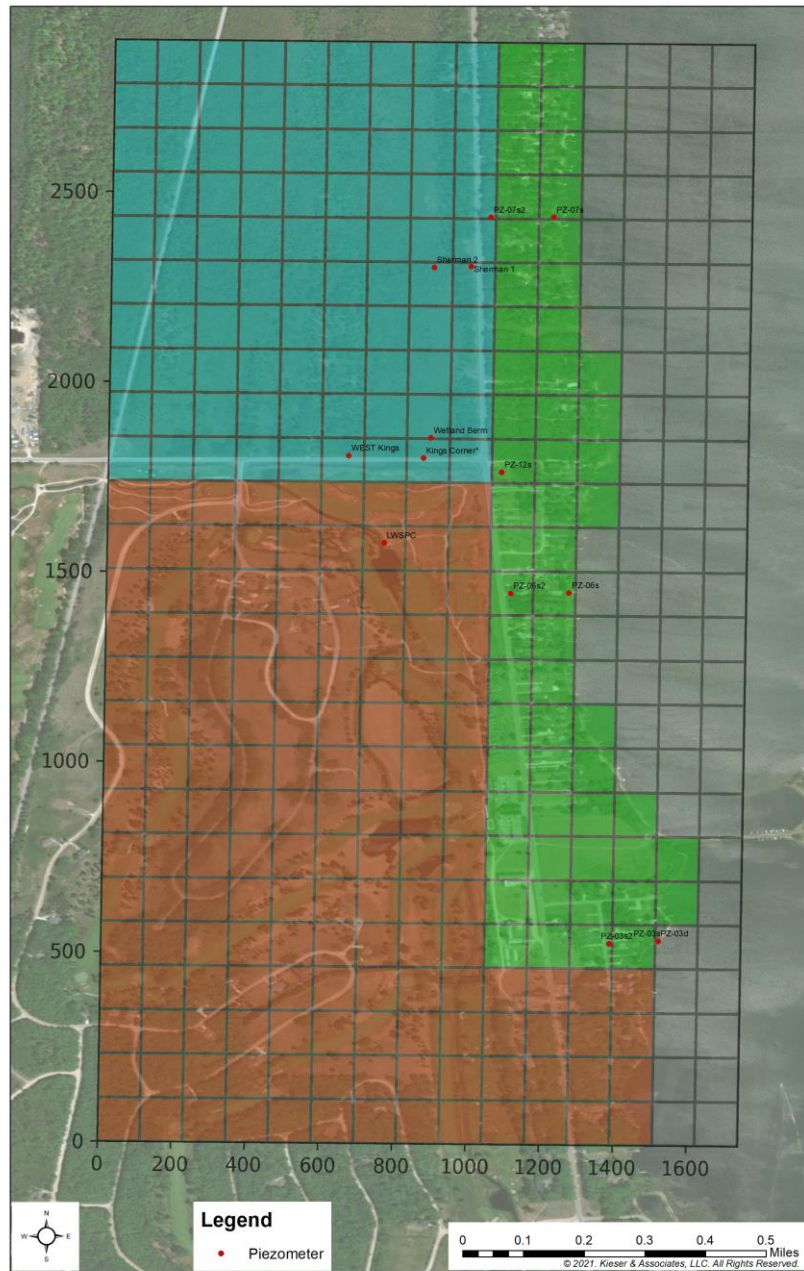
Figure 1 - MODFLOW grid and input piezometer locations overlaid on Cedar Lake topography. Shading represents the different regions the model output grouped for spatial analysis: teal represents the northwest wetland, green represents the groundwater contributing areas of the shoreline, and red represents the non-contributing region where groundwater does not move to Cedar Lake via groundwater directional flow or via surface water.
