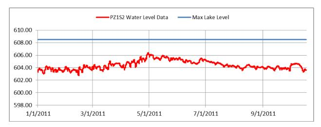
PZ1S2 is a second shallow piezometer located at this property. It is installed approximately 200 feet back from the lakeshore.
