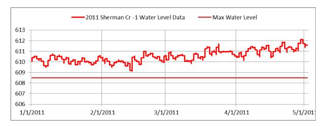
Sherman Cr-1 is a shallow piezometer. It is located within the Cedar Lake Rd easement and was removed in May of 2011 because of the improvement work on Cedar Lake Rd. The piezometer was reinstalled in October 2011.
