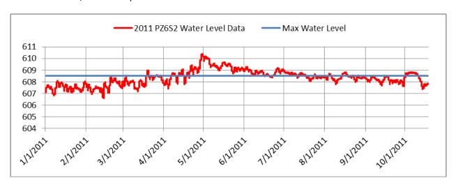
PZ6S2 is a second shallow piezometer located at this property. It is installed approximately 200 feet back from the lakeshore.
