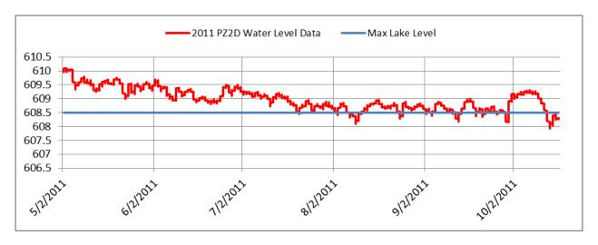
PZ2D is a deep near shore piezometer. It is installed immediately adjacent to PZ2S.
