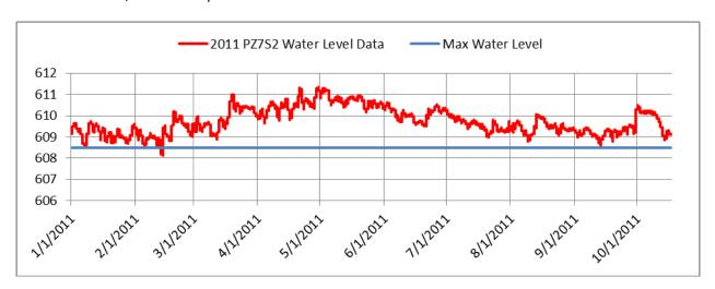
PZ7S2 is a second shallow piezometer located at this property. It is installed approximately 200 feet back from the lakeshore.
