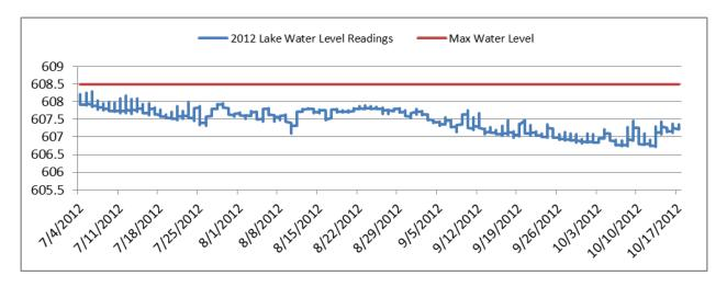
The outflow piezometer is located in the lake. It is unique to the rest of our piezometers, as it is not used to measure ground water movement. It functions as an automated staff gauge, recording the lake's water level readings.
