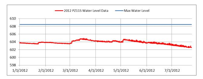
PZ11S is a shallow piezometer. The datalogger was re-deployed in July of 2012 incorrectly after it was pulled to collect data, hence, no data collected in 2012 beyond July. It was re-deployed properly in October 2012. So, data is once again being collected.
