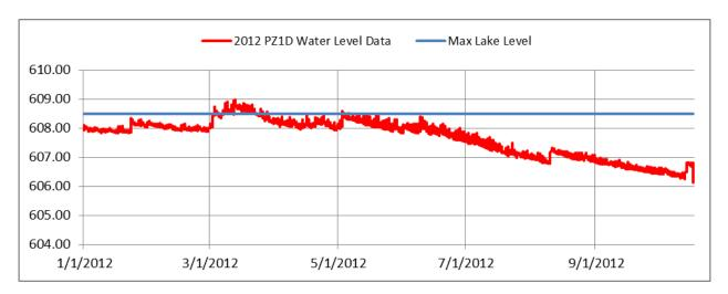
PZ1D is a deep, near shore piezometer. It is located immediately adjacent to PZ1S. The screen of the deep piezometer (PZ1D) is approximately always 8 feet deeper than the screen of the shallow piezometer (PZ1S).
