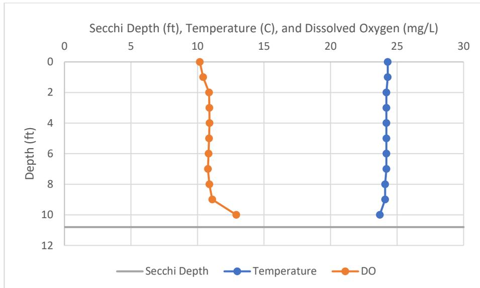
Figure 2 – Early-season survey (July 1, 2021) dissolved oxygen and temperature profiles with Secchi depth, taken at the deepest point in the lake.
