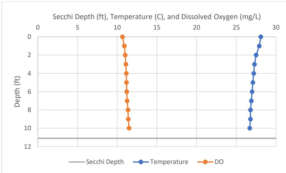
Figure 3 – Late-season survey (August 25, 2021) dissolved oxygen and temperature profiles with Secchi depth, taken at the deepest point in the lake.
