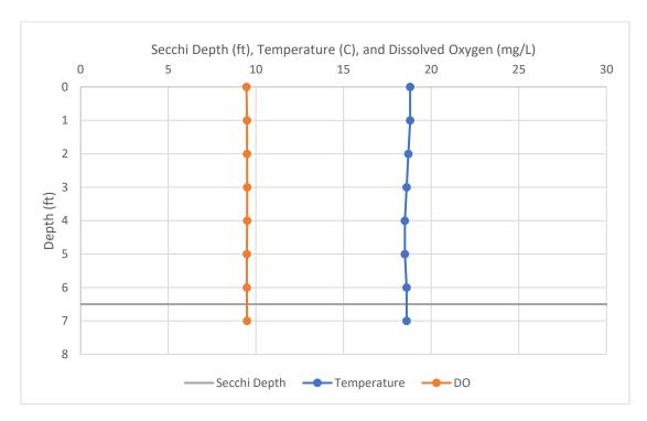
Figure 3 – Late-season survey (August 29, 2023) dissolved oxygen and temperature profiles with Secchi depth, taken near AROS 470.
