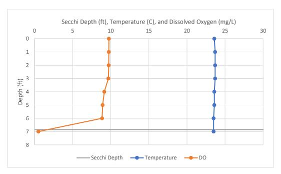
Figure 2 – Early-season survey (July 10, 2023) dissolved oxygen and temperature profiles with Secchi depth, taken near AROS 470.
