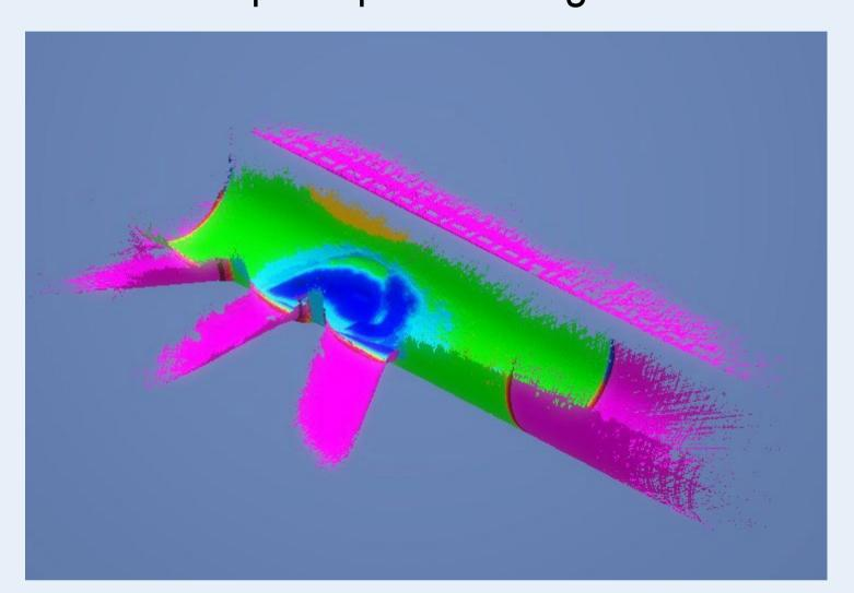
A vessel surface reconstructed from multiple scans after assessment.
