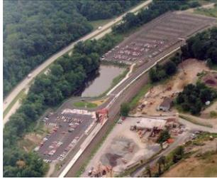
**Cortlandt Station**, Cortlandt, New York. Planning and design for new train station parking and site access, including a 750-car parking lot, road access system, accessible parking, and intermodal transfer for buses and taxis at new station for Metro-North Railroad. Planning included environmental impact statements, landscaping, traffic and road design, as well as complete design of parking lot.
