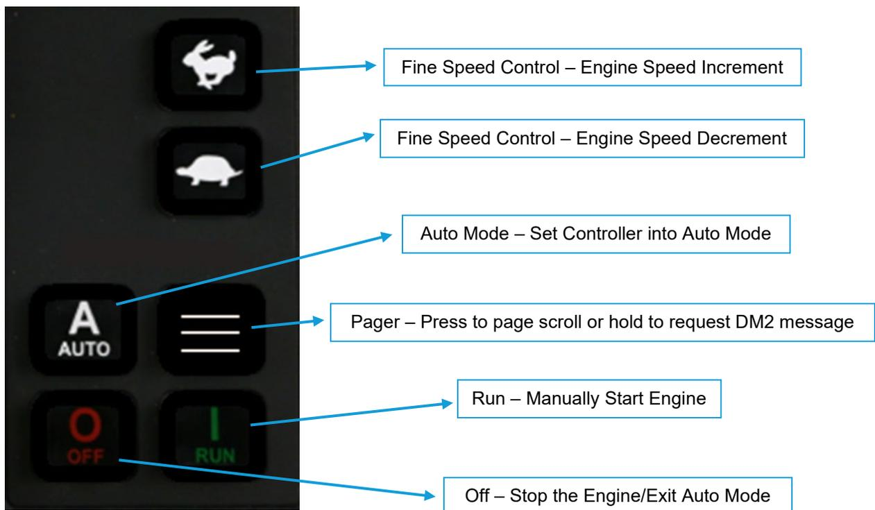
**Figure 11: Controller Button Descriptions**
