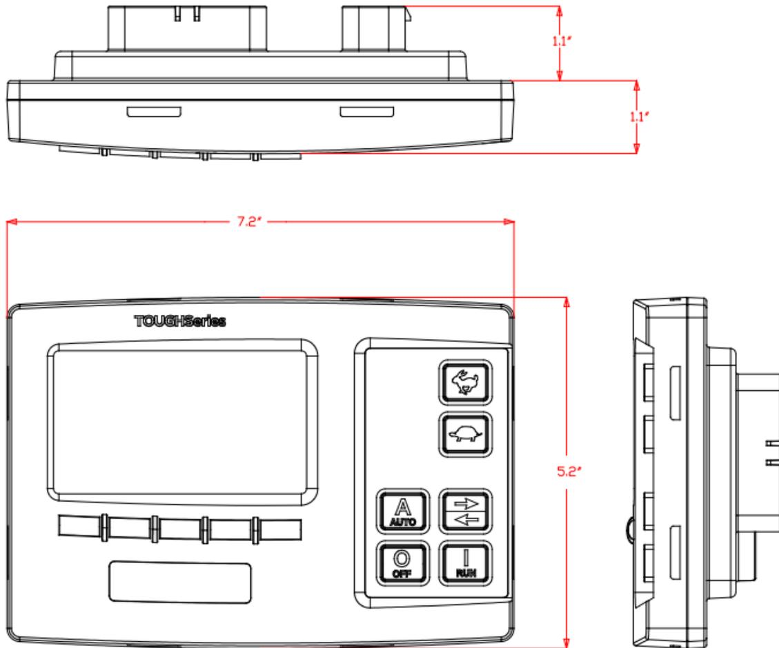
**Figure 2: Controller Dimensions**
