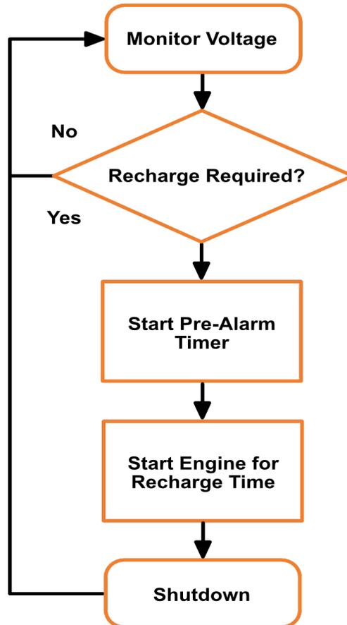
**Figure 19: Battery Recharge Functionality**
