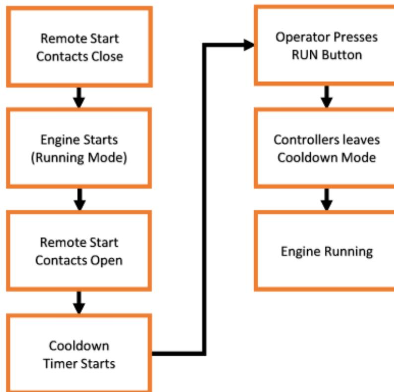
**Figure 15: Cooldown Functionality**
