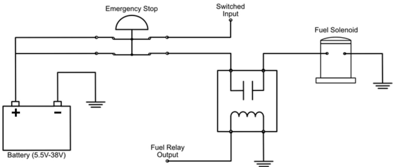
**Figure 6: Emergency Stop Wiring Diagram**
