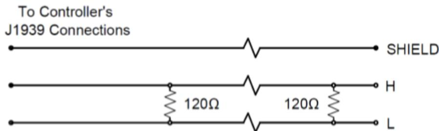
**Figure 8: Communications Wiring**
