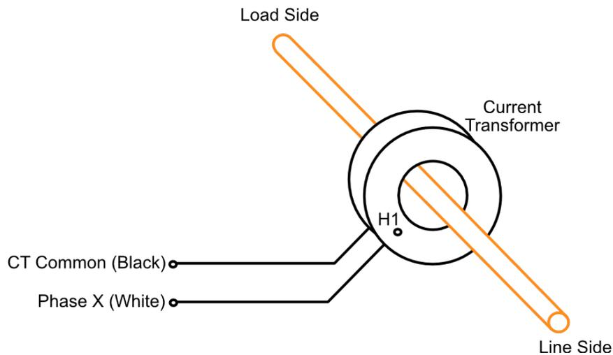
**Figure 10: CT Wiring**
