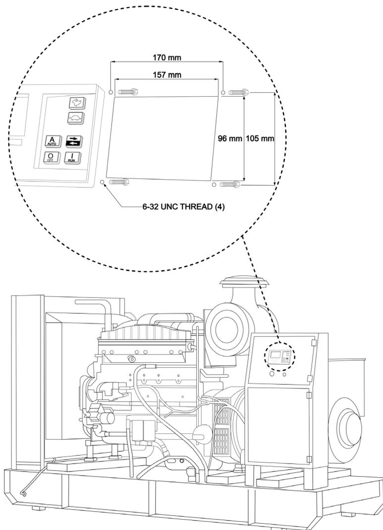
**Figure 1: Mounting Cut-Out**
