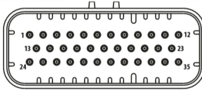
**Figure 4: Auxiliary Connector – J2 (AMPSEAL 35-pin)**
