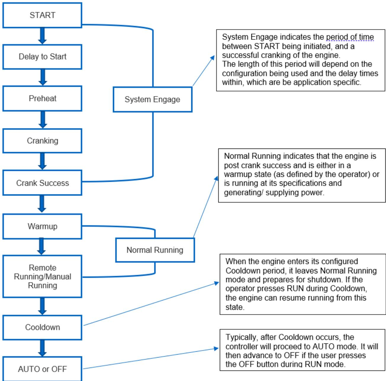
**Figure 16: Flow of Active State**
