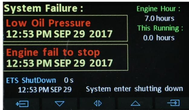
**Figure 18: Failure State**
