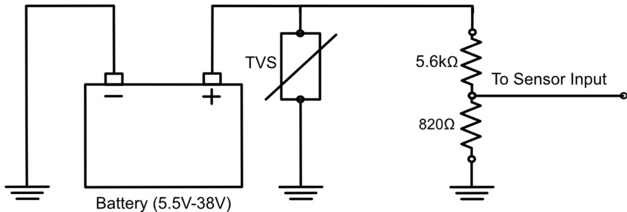
Figure 7: Universal Sensor Wiring Example
