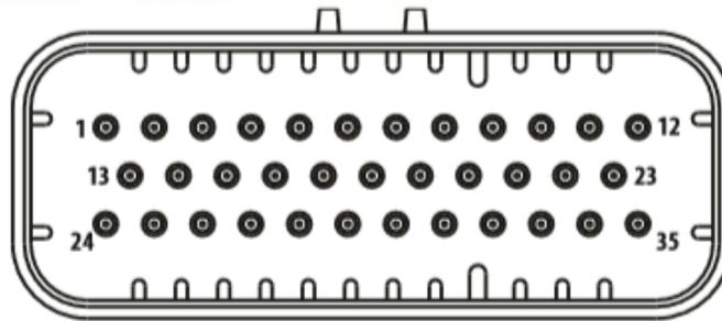
**Figure 3: Main Connector – J1 (AMPSEAL 35-pin)**
