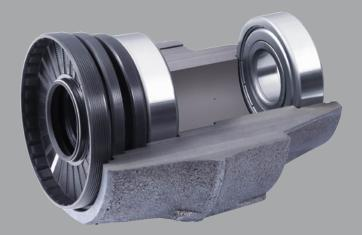
Encore washers are built with **two commercial grade SKF bearings**. These premium bearings are sealed for maximum protection leading to longer life with fewer repairs. The three individual seals with 5 lips provide a water-tight barrier around the drive shaft to protect the bearings from damaging moisture. To ensure better performance, the durable AC motor has no brushes.
