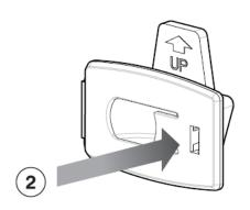
2. Press the outside door until it rotates all the way in and locks into place.
