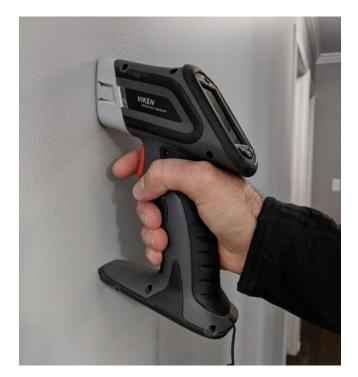
Example of lead XRF instrument.
