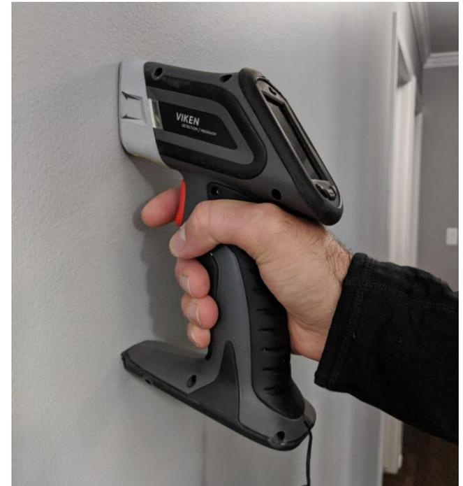
*Example of lead XRF instrument.*
