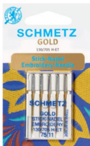
**System 130/705 H-ET** with light ball point, enlarged eye and titanium-nitride coating, which provides a longer service life in applications with a high number of stitches and less residues on the needle; for embroidery and tough, densely woven materials
