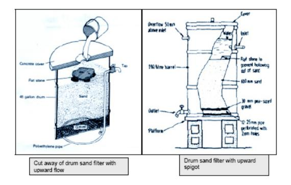
Figure 1. Sand-in-a-barrel filters.
