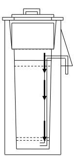
Figure 5. Cross-section of concrete household BioSand Water Filter with INCORRECT standpipe.
