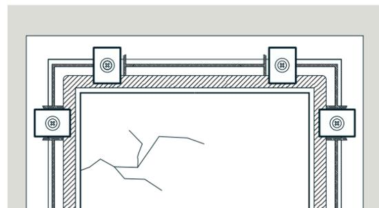
Our replaceable cassette system means that in the event of breakage, or if your glass unit breaks down and becomes misty, you can simply and easily change the glass without replacing the door.
