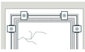
Our replaceable cassette system means that in the event of breakage, or if your glass unit breaks down and becomes misty, you can simply and easily change the glass without replacing the door.
