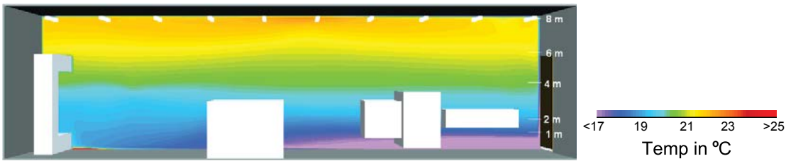
Room pre Airius installation
