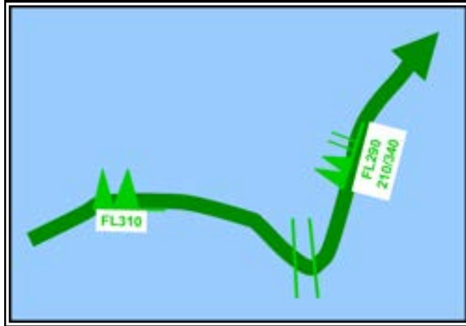
Forecast maximum speeds of 100 kt at FL310 at one location and 120 kt at FL290 at another location. At the latter location, the base of the 80-kt wind field is FL210, and the top of the 80-kt wind field is FL340.
