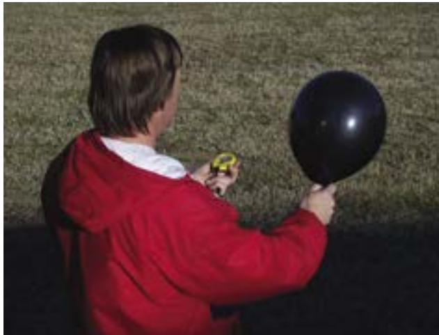
Figure 3-2. Preparing to release a pibal.
