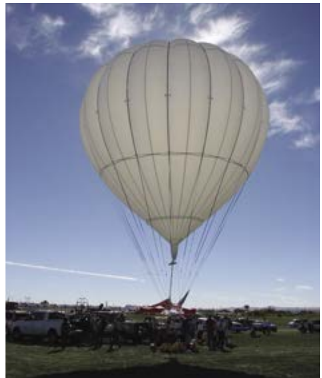
Figure 11-3. Quick fill design gas balloon.
