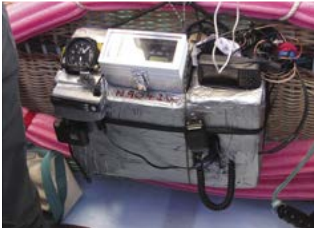
Figure 11-6. Instruments and radios are sometimes carried in a pod such as this.
