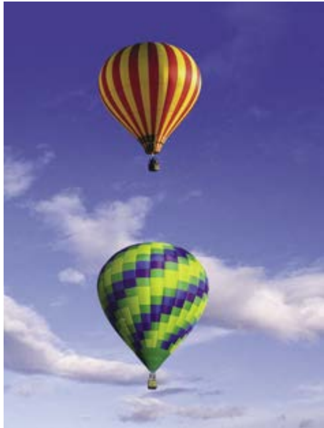
Figure 6-15. The balloon below has the right of way while ascending. The pilot of the higher balloon should, as a courtesy and in the interest of safety, yield the right of way to the ascending balloon, as that pilot is probably unable to see the balloon above.
