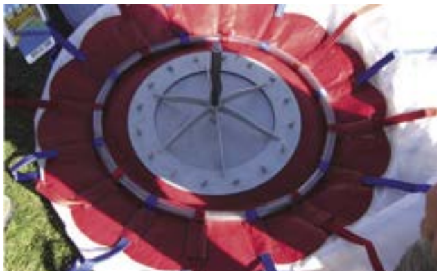
Figure 11-4. Maneuvering valve on quick fill gas balloon.
