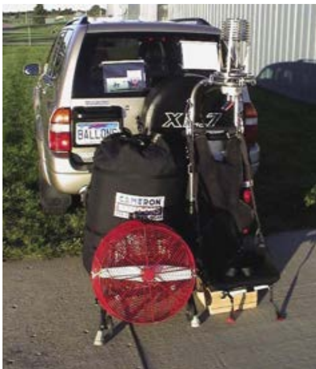
Figure 2-13. This is an example of a transport vehicle which carries a small balloon, three adults, a 20-inch inflation fan, and all other necessary equipment.
