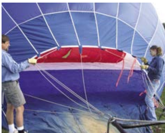
Figure 6-14. Determining correct inflation fan placement. Note that the strips of tape are generally pointing into the mouth. In this case, the pilot would do well to incline the fan slightly towards the right side of the mouth, in order to better “seal” the envelope opening, and get a more efficient inflation.
