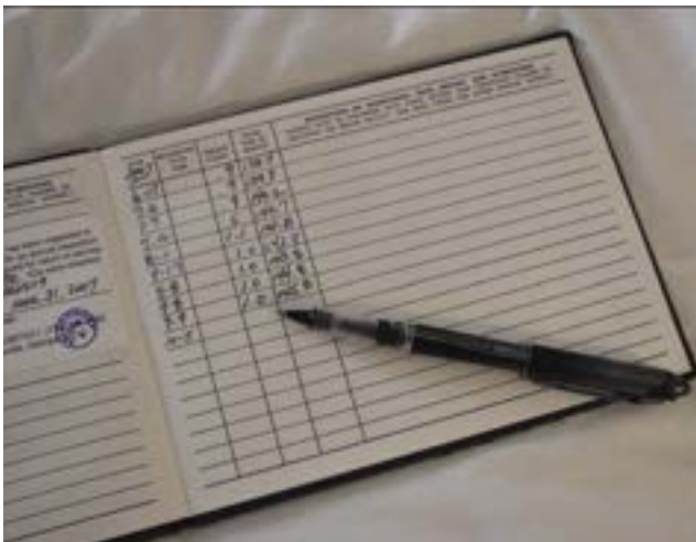
Figure 8-13. Aircraft log books or maintenance records are for aircraft time and not for passenger names and flight experiences.
