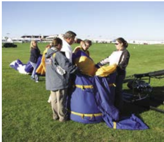
Figure 8-11. Packing the balloon. This pilot has elected to position the envelope bag near the basket and is bringing the balloon to the bag, rather than picking up the bag each time to move it towards the basket. Some pilots prefer this method, as it means less lifting for the crew.
