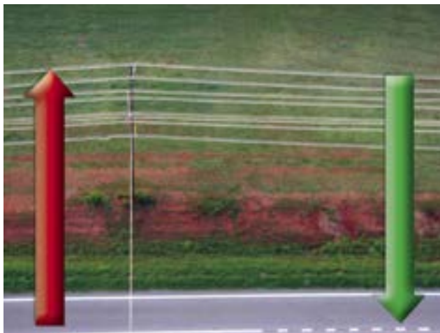
Figure 7-10 The movement of the power lines either up or down in the pilot's field of vision can indicate whether or not the balloon has sufficient obstacle clearance.
