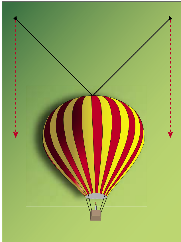
Figure 6-6. Double crown lines forming a 90° or wider angle offer the greatest inflation stability provided crew walk them directly upwind on stand-up.
