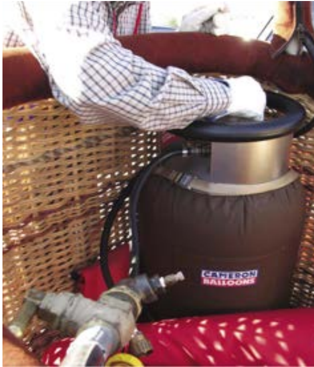
Figure 8-12. Refueling. Note that this pilot is exercising safety precautions with sleeves down and gloves on.
