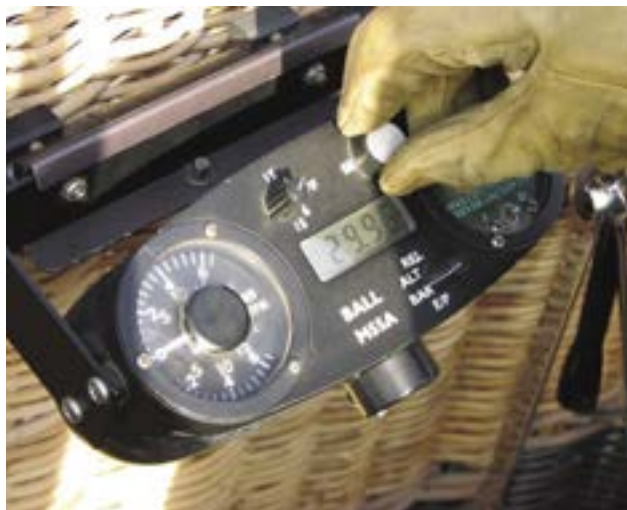
Figure 6-10. The altimeter should be set to barometric pressure, if available, or to the field elevation.
