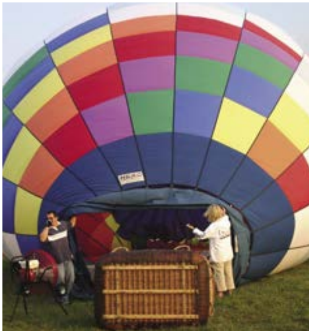
Figure 2-12. Balloon inflation using a typical inflation fan.
