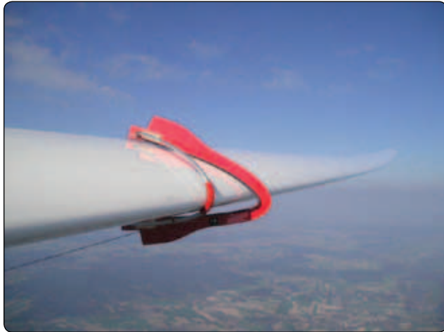
Figure 2-3. Mechanical bug wipers can be installed to slide back and forth along the leading edge of the wing.
