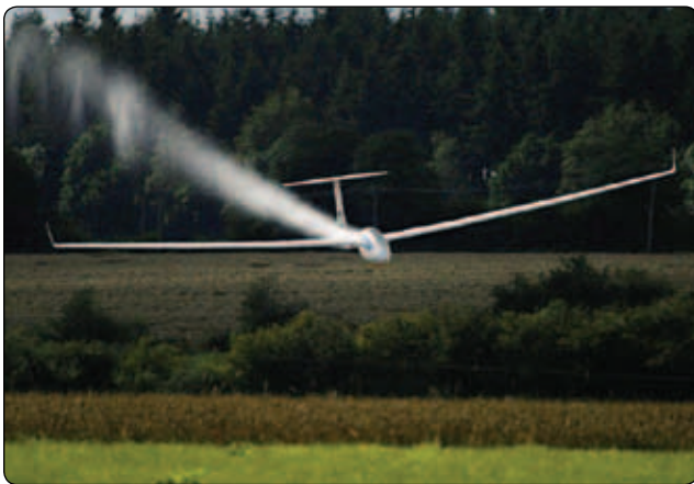
Figure 2-4. Sailplane dropping water ballast before landing.
