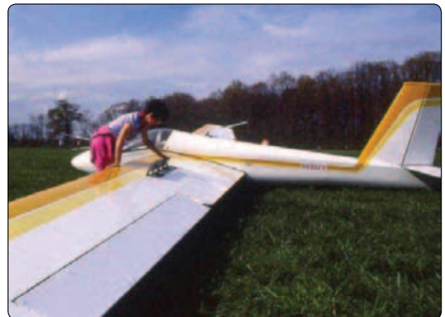
Figure 6-14. Positive control check of spoilers.
