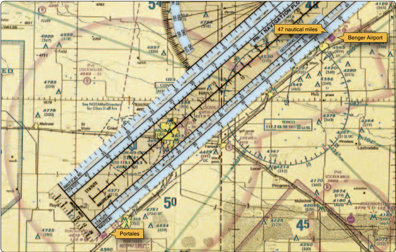
Figure 11-5. Measuring distance using the navigation plotter.
