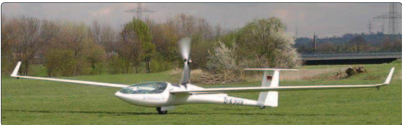
Figure 2-16. A DG-808B 18-meter high-performance glider in self-launch.
