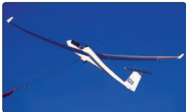
Figure 2-2. Schmepp-Hirth Ventus-2 glider with factory winglets installed.
