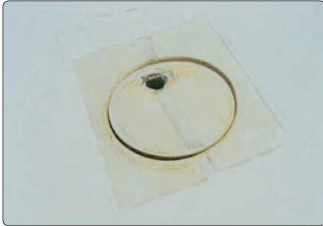
Figure 5-21. Water ballast tank vented filler cap.
