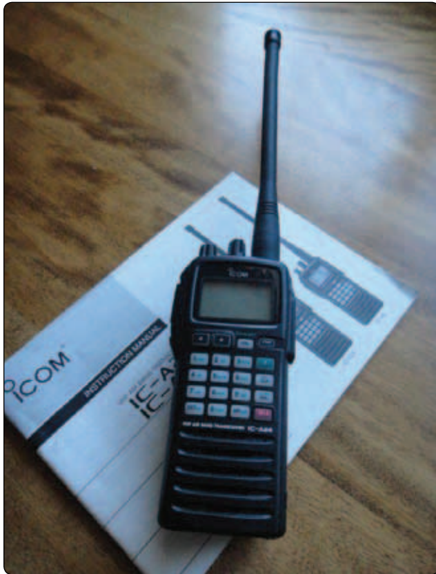
Figure 12-16. On a cross-country tow, the tow pilot and glider pilot should have two way communication using portable radios.
