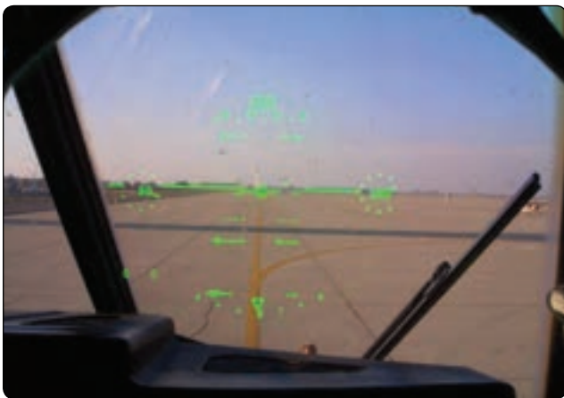
Figure 5-13. HGS using a holographic display.
