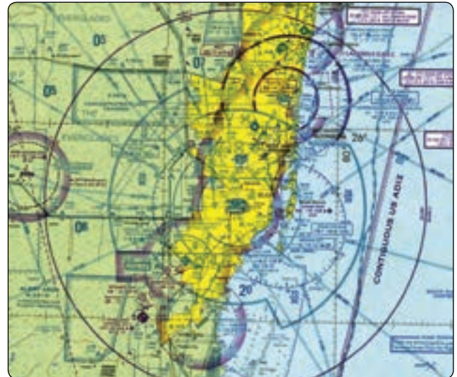
Figure 5-32. Temporary flight restriction (TFR).
