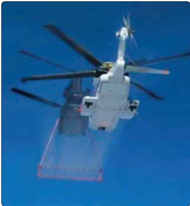
Figure 7-1. Icing tests. To safely provide an all-weather capability and flight into known icing conditions that would otherwise delay or cancel winter flight operations, the digital control of the S-92 Rotor Ice Protection System (RIPS) determines the temperature and moisture content of the air and removes any ice buildup by heating the main and tail rotor blades. The system is shown here during testing.
