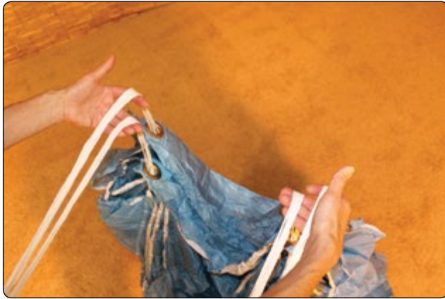
Figure 5-117. Push the slider up to the slider stops.
