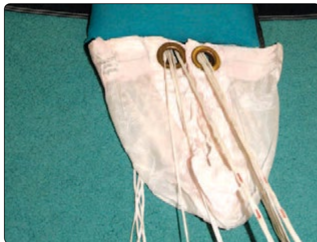
Figure 5-72. Pull slider down.
