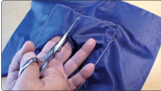
Figure 7-32. Wear the damaged parachute as if it were a mitten while cutting and you will not cut the patch that was just carefully placed.
