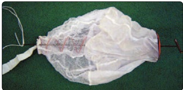
Figure 5-108. Gun rod through the pilot chute.
