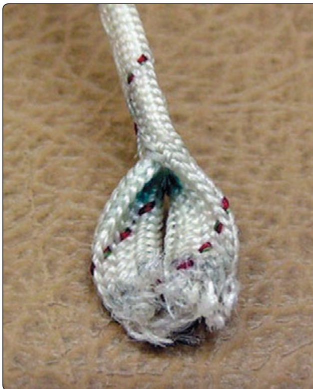
Figure 5-18. Worn closing loop.
