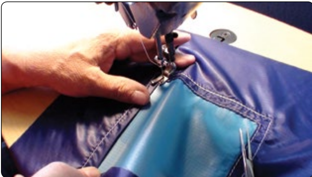
Figure 7-27. Correct fold corner seam.
