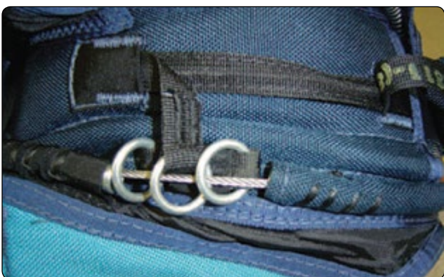
Figure 2-58. Ripcord cable routing through rings.
