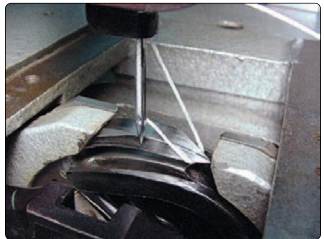
Figure 6-70. Second step in forming a stitch.
