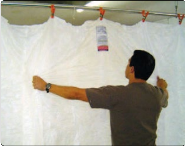
Figure 5-20. Ram-air canopy hanger—top skin inspection.
