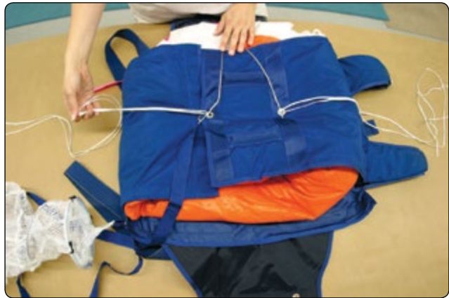
Figure 5-61. Upper temp pin seated.
