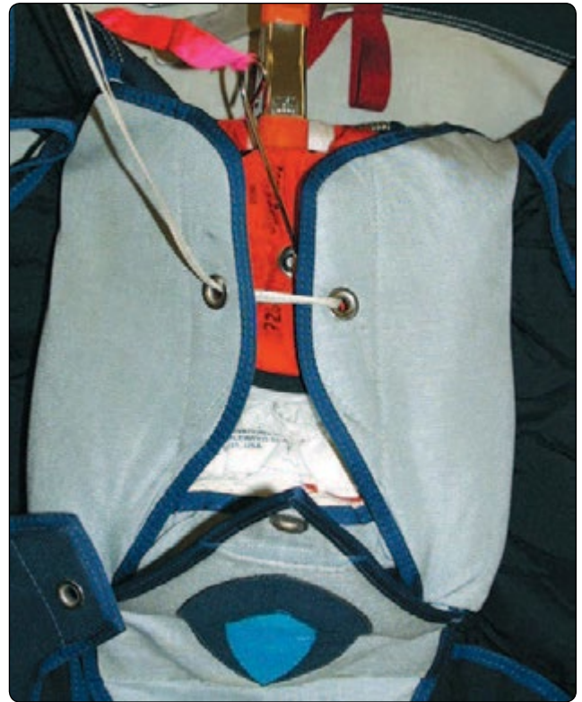
Figure 5-111. Close right and left flaps simultaneously.
