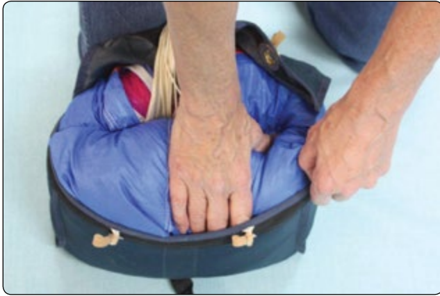
Figure 4-27. Shove the canopy down into the bag filling the corners.
