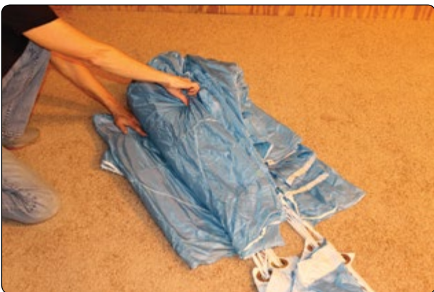
Figure 5-124. If the PRO packed canopy was laid down carefully, it will be essentially flaked. Only minor straightening is necessary.
