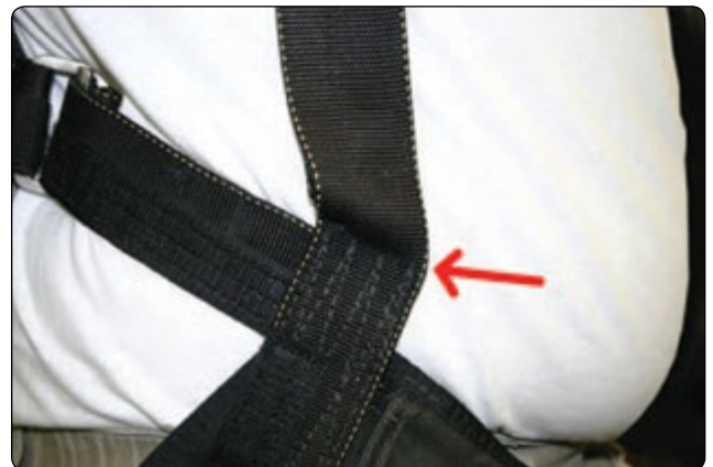
Figure 2-18. Stair-stepped harness (aka stepped harness) junction warping.
