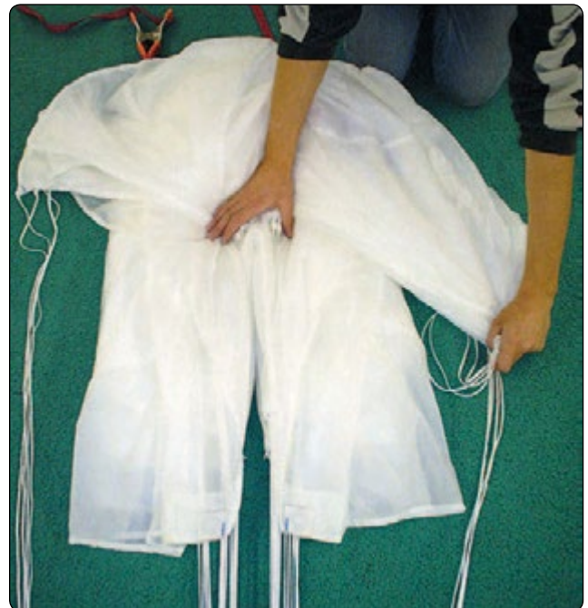
Figure 5-83. Pull down the trailing edge.
