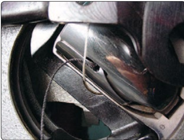
Figure 6-72. Fourth step in forming a stitch.
