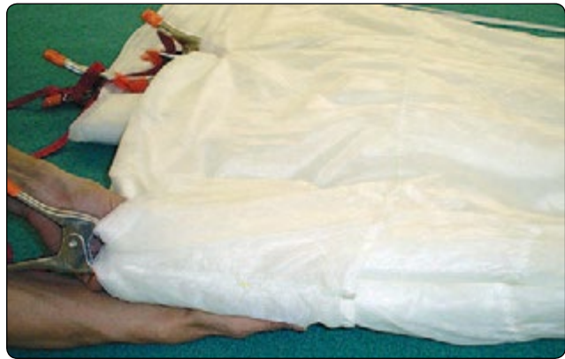
Figure 5-77. Smooth panels under "A" lines.
