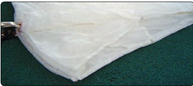
Figure 5-75. Split the leading edge.
