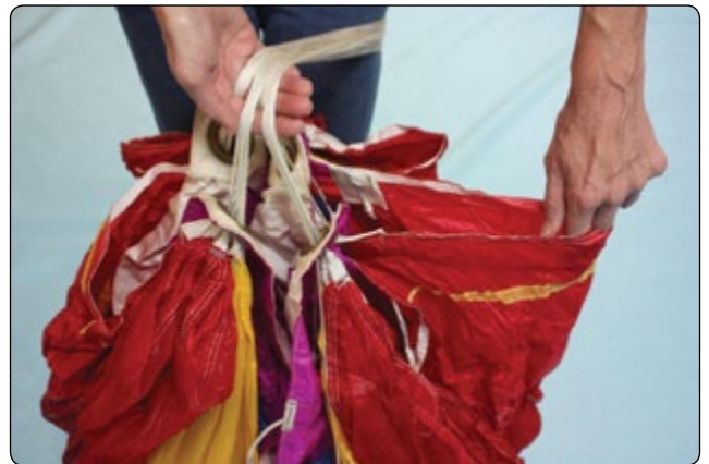
Figure 4-9. Flake the canopy fabric between the A-B, B-C, C-D line groups following the perimeter of the canopy.
