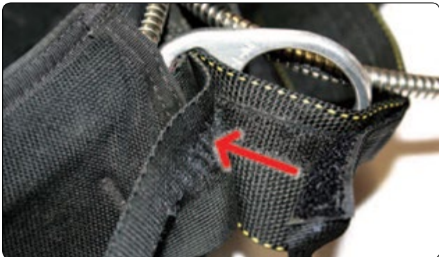
Figure 2-56. RSL Velcro riser damage.
