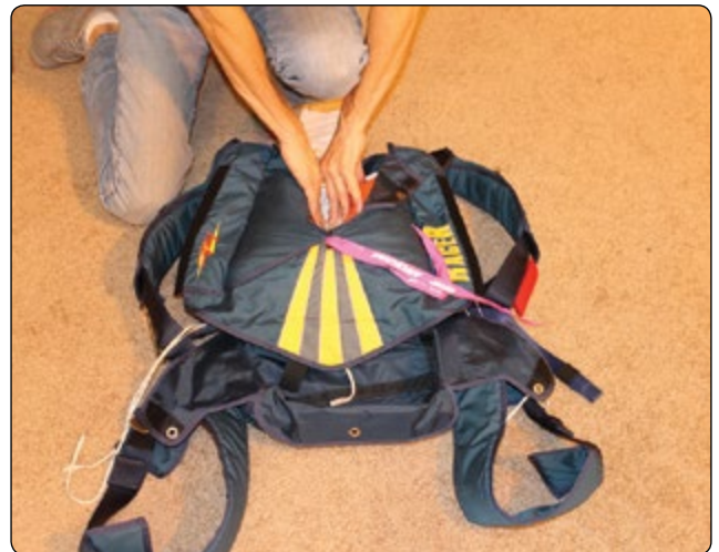
Figure 5-151. Maintain the division of the canopy by pushing the ears down and outward. This is where the pilot chute spring will nest.
