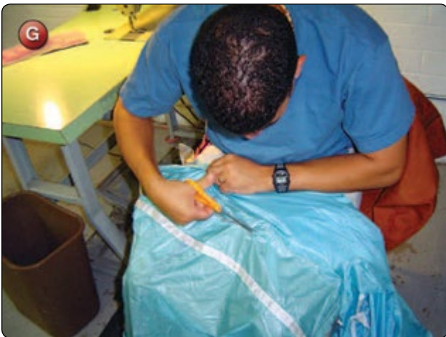
6. Turn the panel inside out. Trim the damaged panel at .62 inch from the edge of the panel edge. [Figure G]
