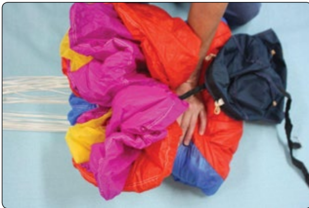
Figure 4-23. Make an additional “S” fold.
