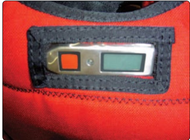
Figure 2-47. CYPRES® control unit vinyl pocket.
