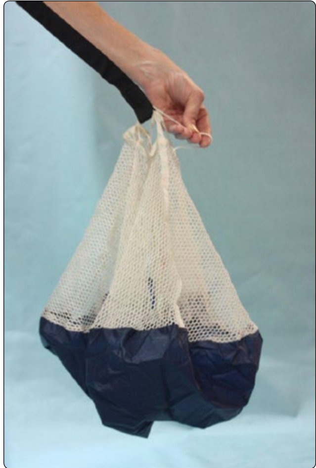
Figure 4-35. Drop the excess line into the pilotchute.
