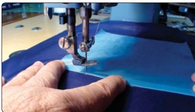
Figure 7-18. Start patch to damage.
