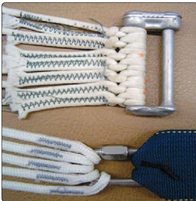
Figure 5-13. Connector link line attachment methods.
