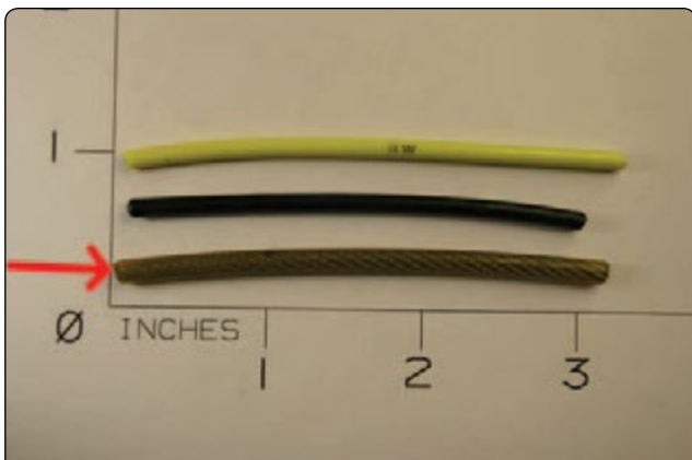
Figure 3-101. 7x7 stainless steel corrosion resistant cable.
