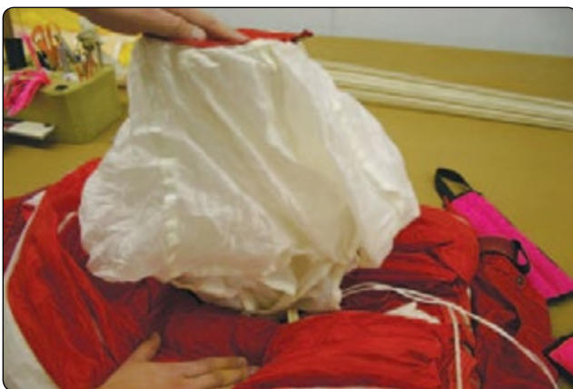
Figure 4-55. Type 1 deployment in a pilot emergency rig.
