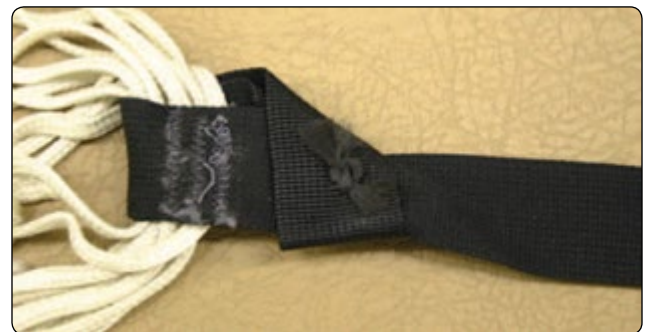
Figure 2-34. Hand tack floating bridle loop.
