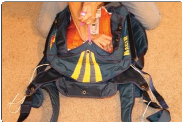
Figure 5-148. Close bottom sub flap.
