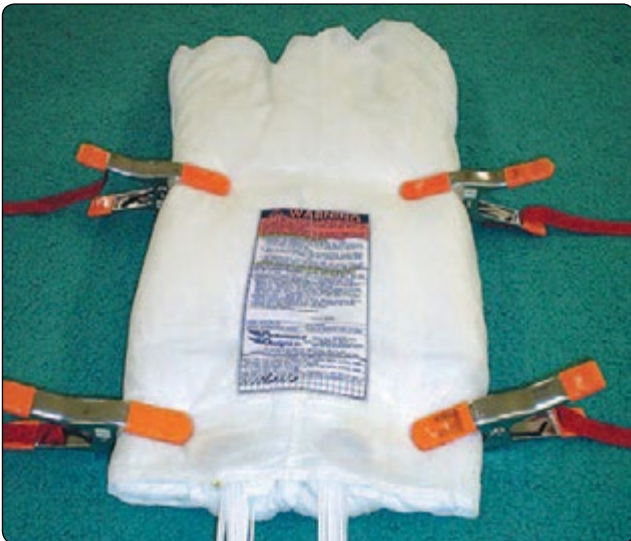
Figure 5-94. Finish wrapping tail, four clamps.
