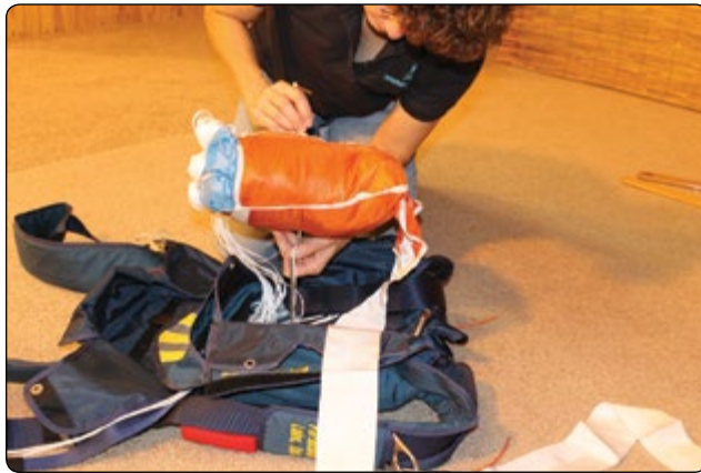
Figure 5-145. A bodkin that has been pre-loaded through the backpad of the container can now be easily pulled through the bag using this second bodkin.
