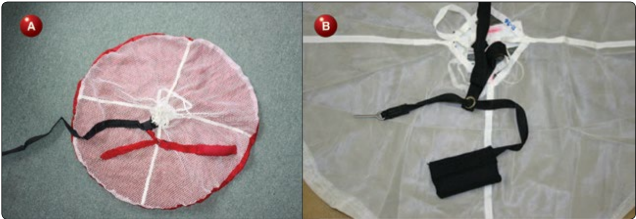
Figure 2-44. A) POP handle with pilot chute and B) POP handle and lanyard.
