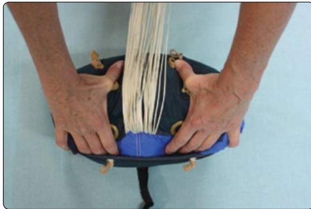
Figure 4-28. Use the flap of the bag to help control the canopy.
