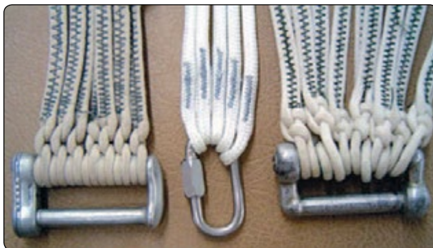
Figure 5-14. Three types of connector links.
