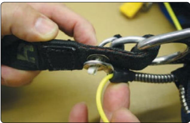
Figure 4-45. 3-ring housing terminal over loop (rear).
