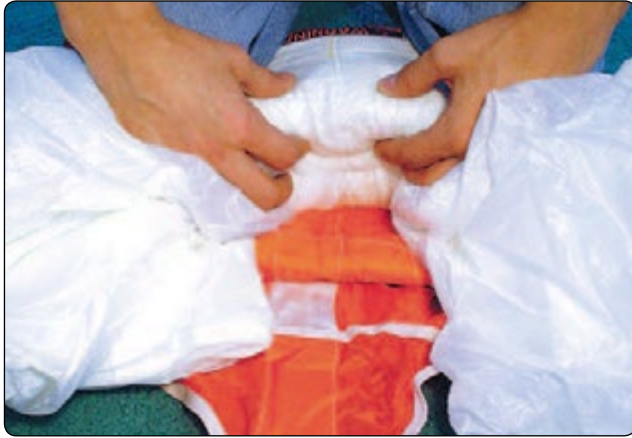
Figure 5-98. Gather and roll center seam fabric.
