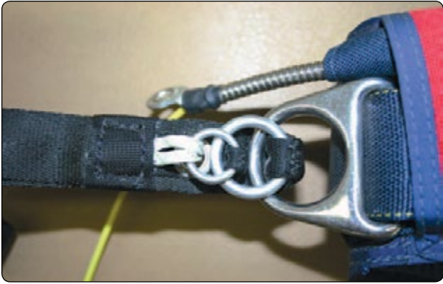
Figure 4-43. 3-ring loop over the top ring.
