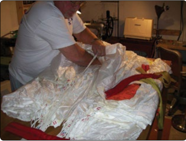
Figure 6-87. A square canopy being packed on a table, which must be accessible from both sides of the table in order to inspect and fold it properly.
