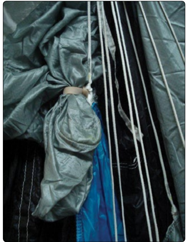
Figure 4-37. Rubber band on center C-Line attachment tab holding apex of slider.
