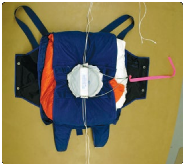
Figure 5-62. Pilot chute seated in position.
