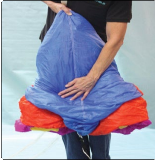
Figure 4-15. Press the air out of the canopy.
