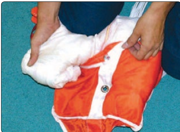
Figure 5-100. Fold molar ends under.
