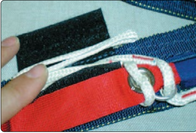
Figure 5-84. Set the deployment brakes.
