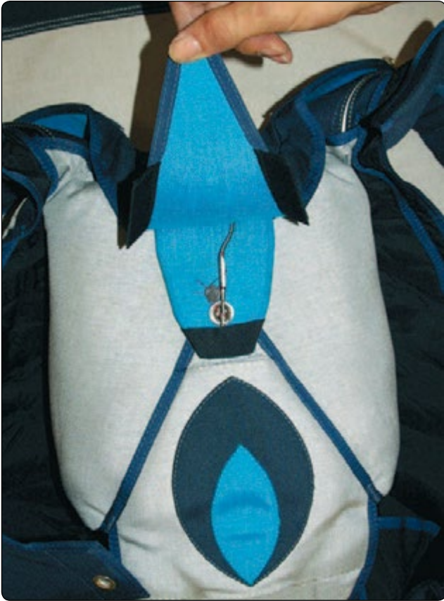
Figure 5-113. Close flap #4 and insert ripcord pin.
