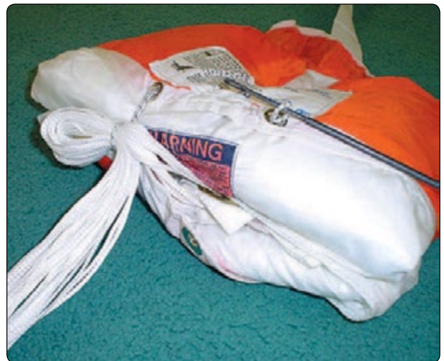
Figure 5-102. Close bag and secure locking stows.
