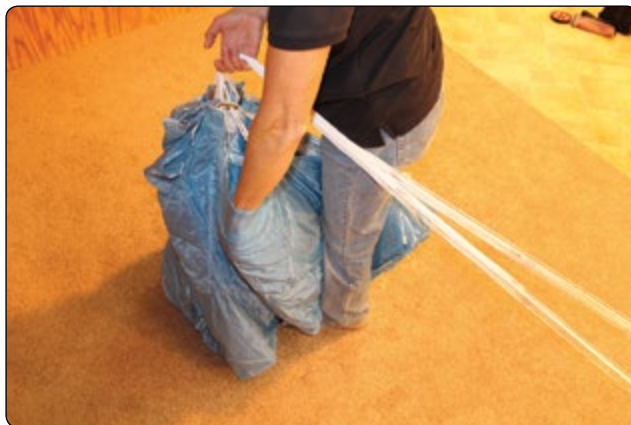
Figure 5-119. Hold all flaked nose cells between the knees. Reach down and flake out material between A/B, B/C, and C/D lines.
