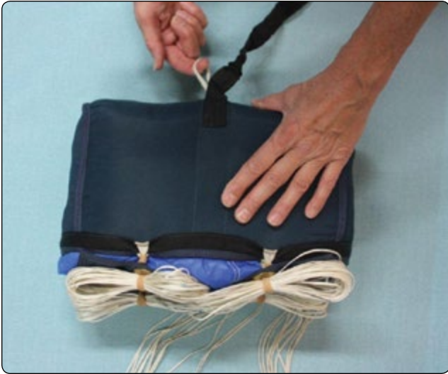
Figure 4-33. Pull pilot chute kill line from bottom of bag.
