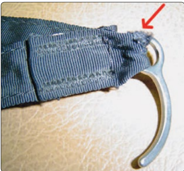
Figure 5-28. TOP bridle with worn pin tape.
