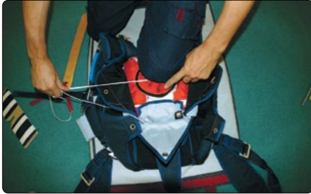
Figure 5-109. Position pilot chute.
