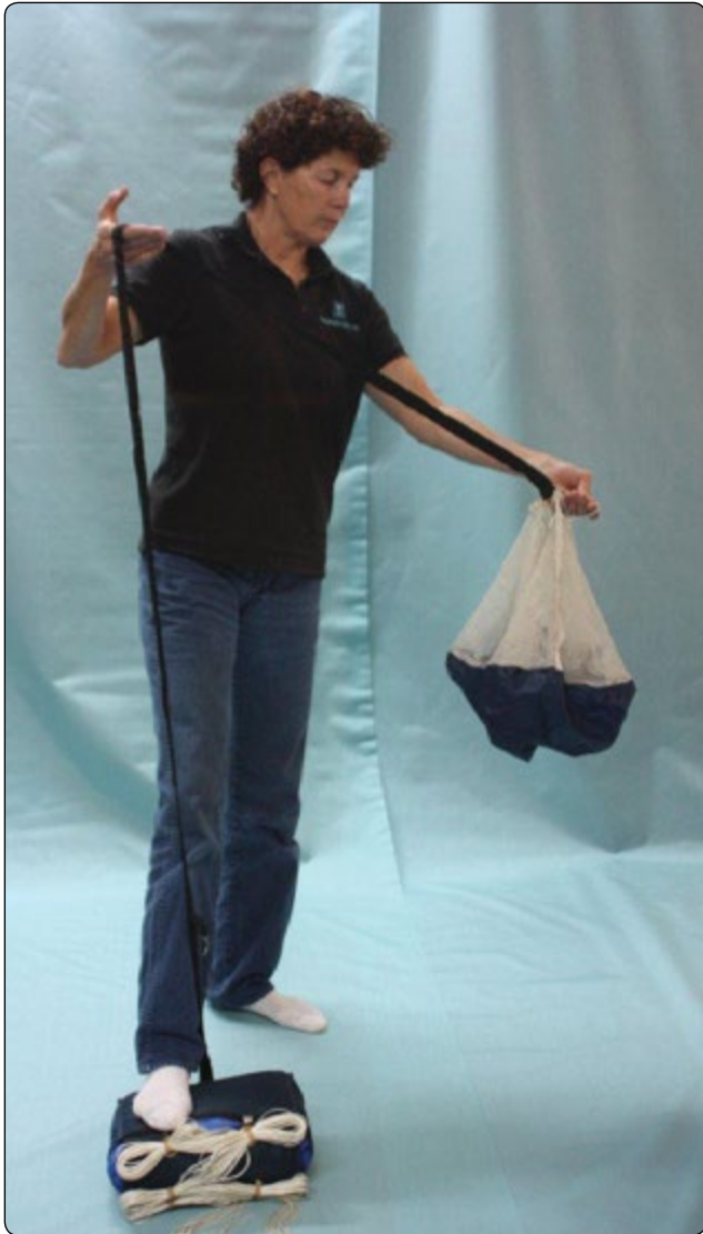
Figure 4-34. Pull the kill line through the bridle.
