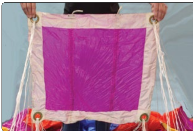
Figure 4-4. Check line continuity and separate line groups. Cock the slider.
