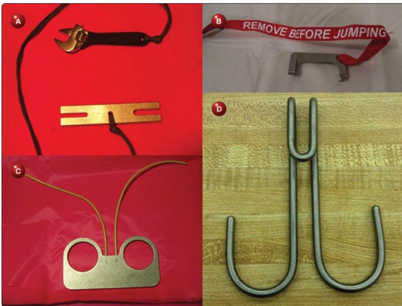
Figure 6-57. (A) link fork, (B) pull check tool, (C) tool used to maintain continuity of risers when removing main parachute from harness, and (D) Pro Pack hook.
