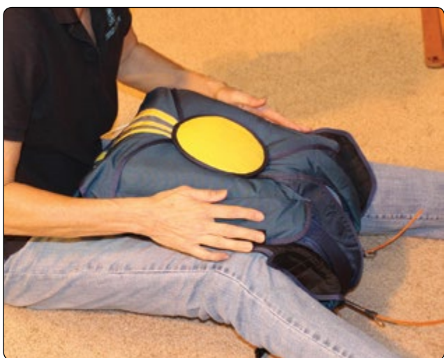
Figure 5-165. Dress per manufacturer’s instructions and attach seal to the last pin.
