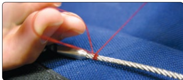
Figure 5-65. Lark’s head the thread on the cable.
