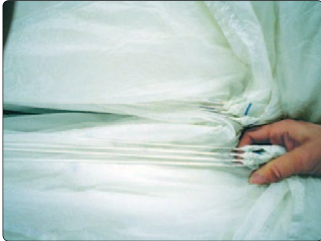
Figure 5-88. Lines are taut in the center.
