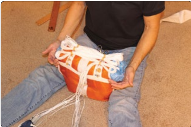
Figure 5-141. Depending on the length of the lines and the width of the bag, all of the rubber bands may or may not be used.
