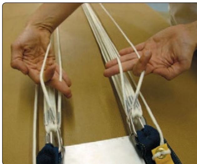
Figure 5-9. Round canopy—four-line check at four-link system.
