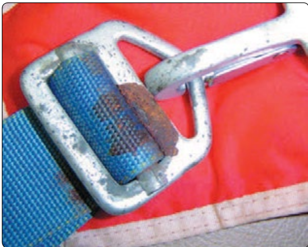
Figure 5-17. Rusty leg snap hardware.
