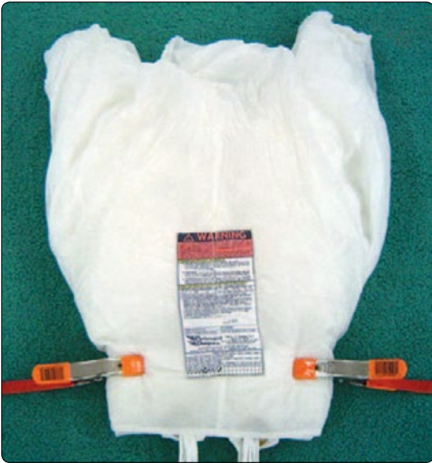
Figure 5-93. Wrap tail, two clamps.
