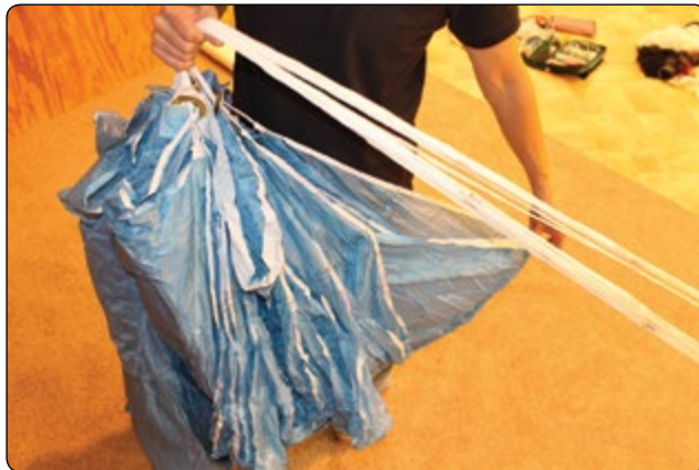
Figure 5-118. Flake the nose cells of the canopy.
