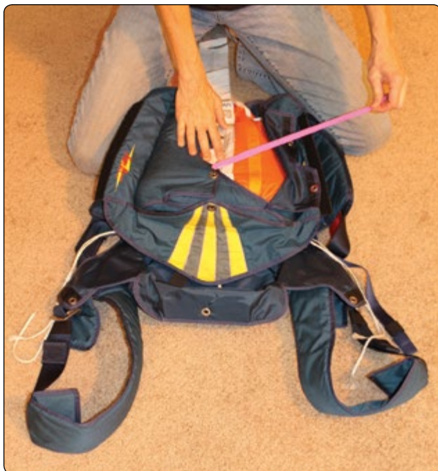
Figure 5-149. Close either side flap (not side-sensitive).
