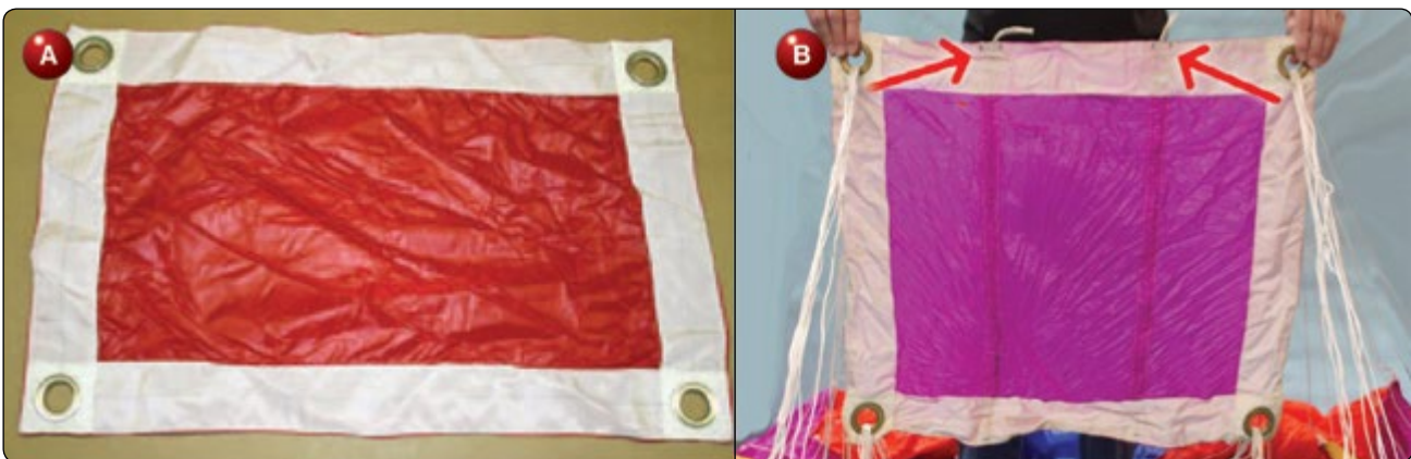
Figure 2-20. A) Non-collapsible slider and B) collapsible slider.
