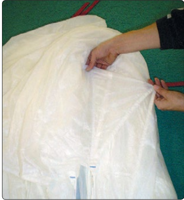
Figure 5-86. Pull stabilizer taut.
