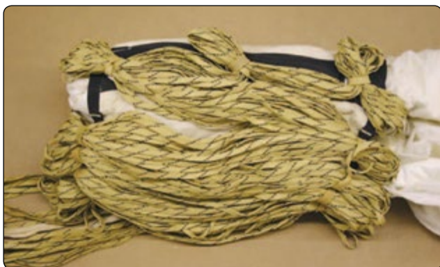
Figure 2-24. Type 4 deployment—Preserve diaper.
