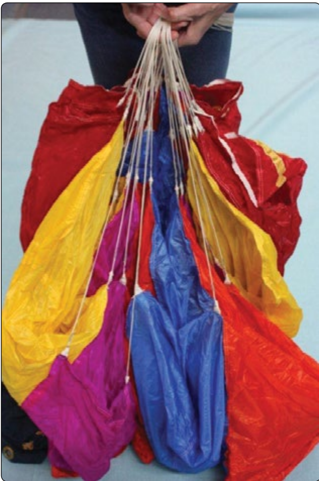
Figure 4-11. Note the staggered order of the line groups. The As are the highest; the Ds are the lowest except for the upper control lines at the very bottom of the picture.
