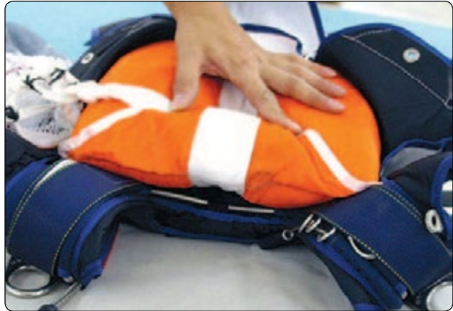
Figure 5-106. Fold the yoke over the bridle.
