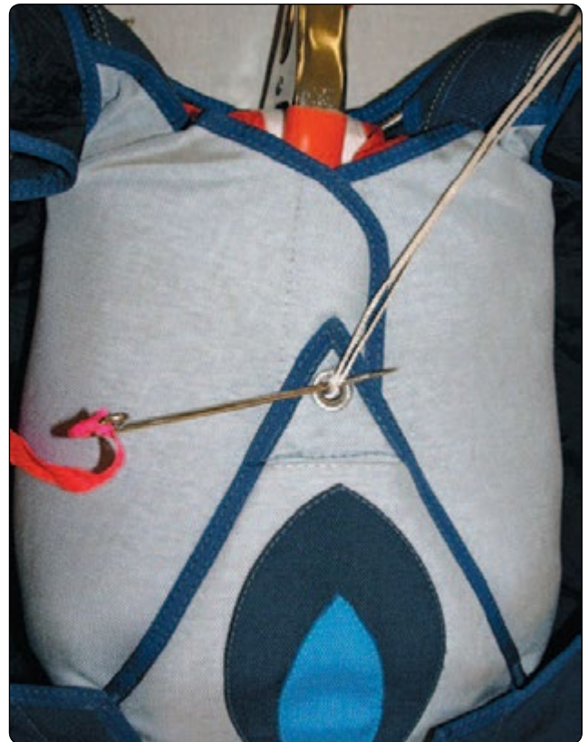
Figure 5-112. Close #3 bottom flap.
