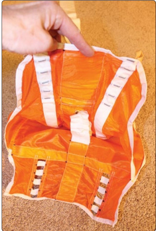
Figure 5-135. Inside the Reserve Speed Bag the buffer tabs form a clear channel for the bottom closing loop.
