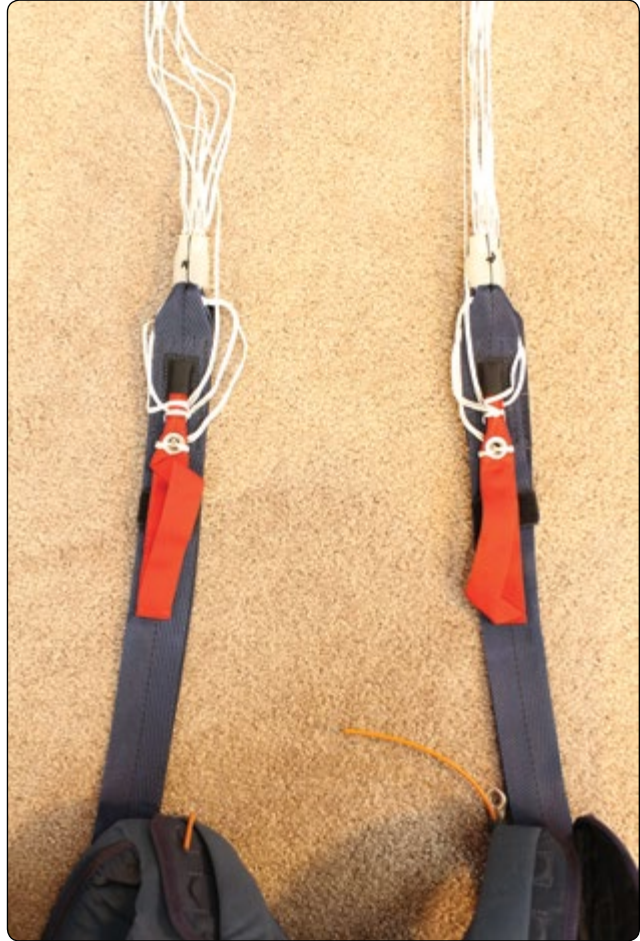
Figure 5-115. Set brakes. Excess lower control line is inserted through top of riser, around nose of toggle, and toggle placed in nose keeper.
