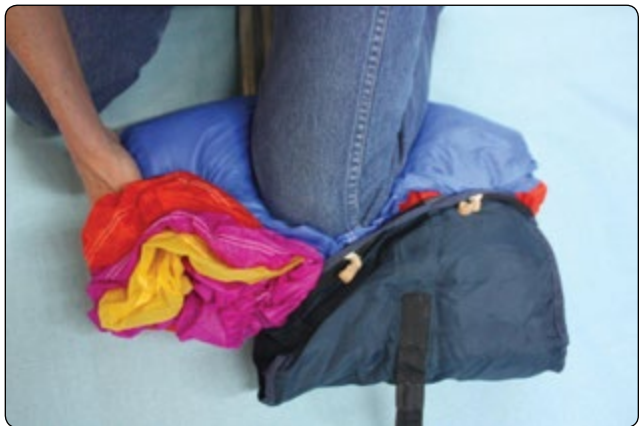
Figure 4-25. Insert the canopy into the bag one side at a time.
