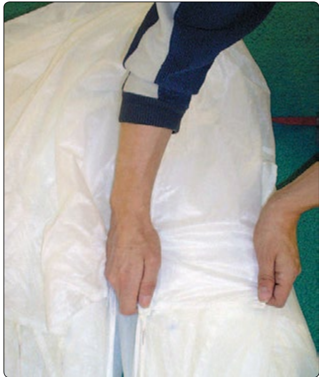
Figure 5-87. Flake the tail.
