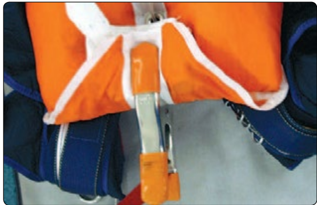
Figure 5-107. Secure yoke/bridle with clamp.
