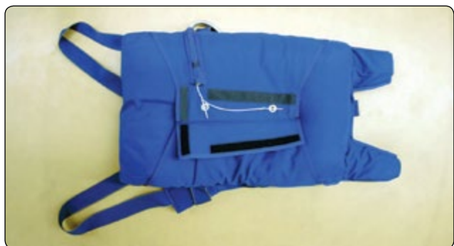
Figure 5-63. Ripcord pins in place.
