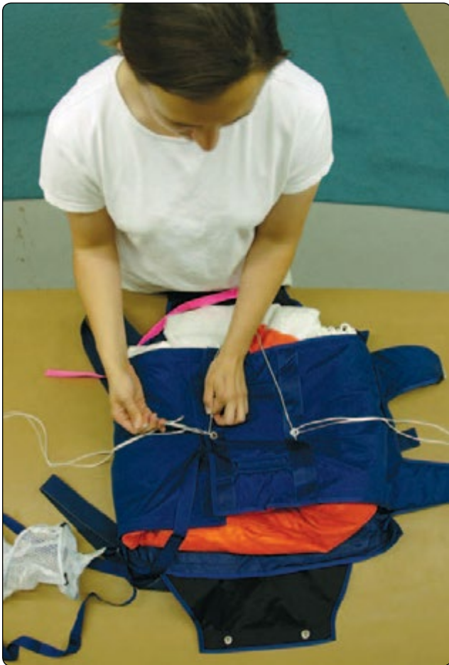
Figure 5-60. Closing bottom flap.
