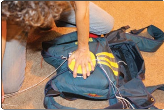
Figure 5-158. Compress pilot chute tucking fabric and mesh between the coils of the spring.
