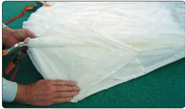
Figure 5-76. Fold half under "A" lines.
