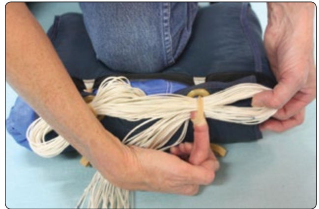
Figure 4-31. The second locking stow. Note the generous size of the bight.
