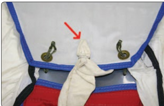
Figure 2-11. Square reserve hesitator loop configuration.
