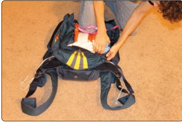
Figure 5-147. Carefully tuck the corners of the bag into the bottom of the container.
