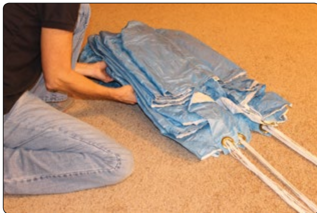
Figure 5-127. Narrow the pack job by folding the divided sections in half. The sections can be folded under or up.
