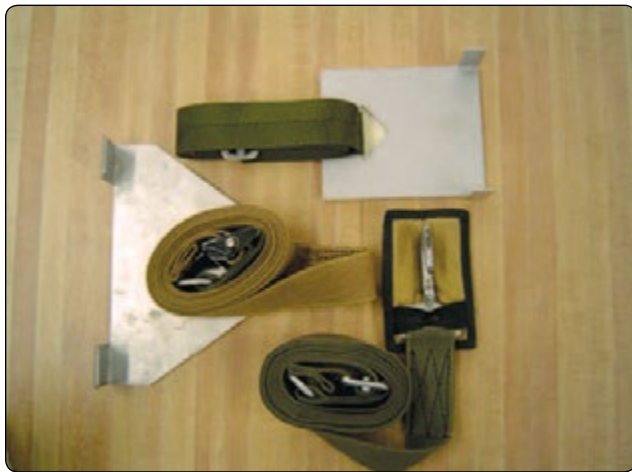
Figure 6-51. Tension board assembly with apex tiedown.
