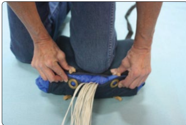
Figure 4-29. The closing flap of the bag is pulled so that the grommets meet the rubber bands. You should not have to stretch the rubber bands very far.
