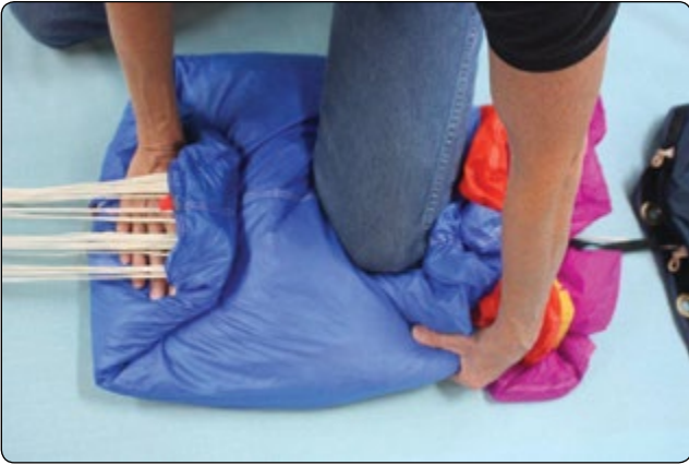
Figure 4-21. Make the first “S” fold.
