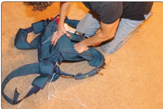
Figure 5-159. Flip the container over and kneel on it to control the spring.
