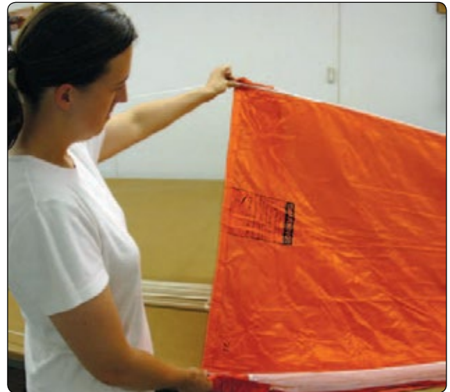
Figure 5-11. Round canopy gore inspection.
