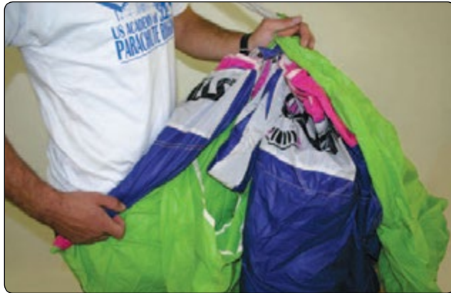
Figure 4-36. Rolling the nose of the canopy.
