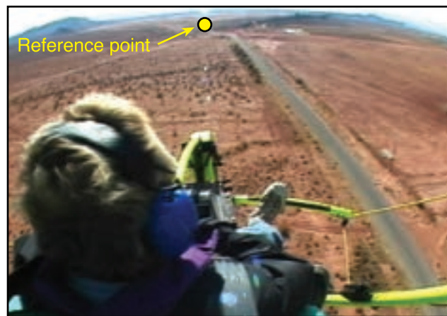
Figure 6-4. Nose reference for straight-and-level flight.
