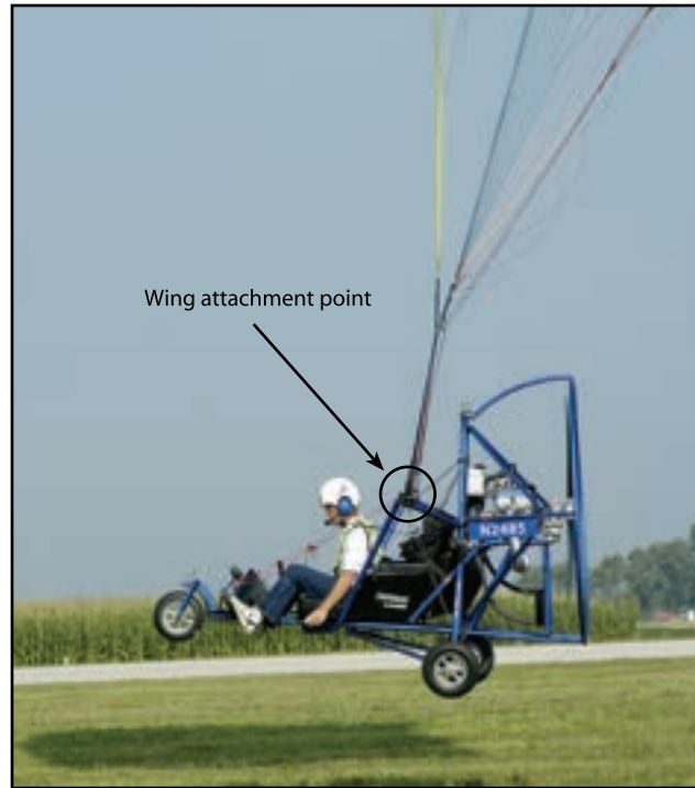
Figure 2-24. Straight and level flight with the nose wheel 7 to 11 inches above the horizontal flight path.
