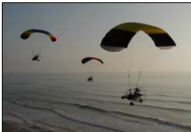
Figure 12-8. You should not fly over water beyond your glide slope to the shore.
