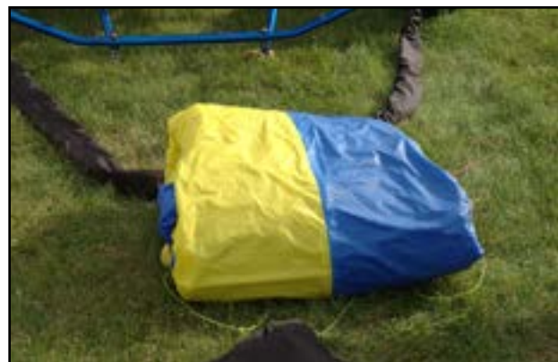
Figure 5-13. Wing removed from wing bag and folded behind the cart.
