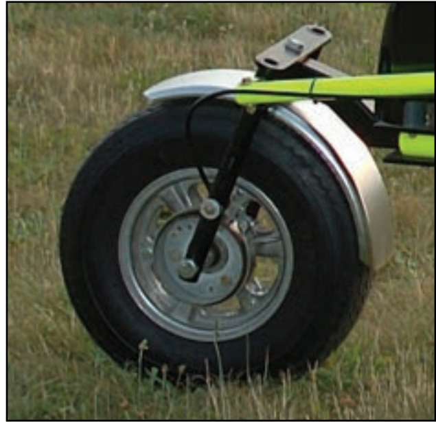
Figure 5-5. Check for proper tire inflation and that the axle bolt is secure.
