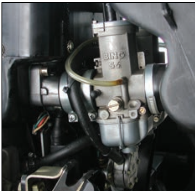
Figure 4-9. Typical 2-stroke carburetor.
