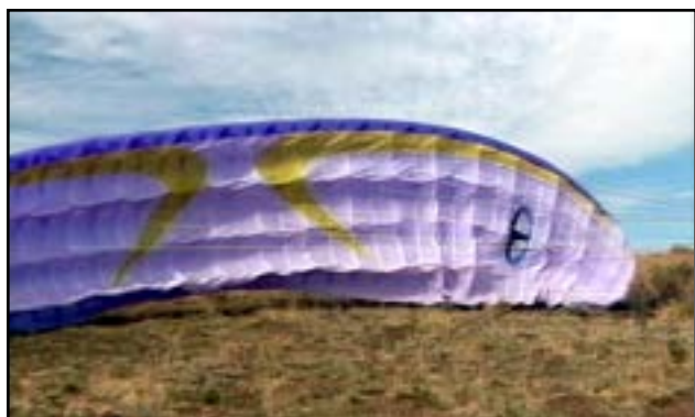
Figure 12-3. A wing wall.
