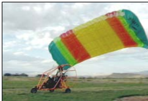
Figure 12-4. A wing lock-out.
