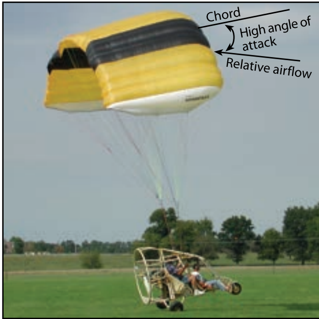
Figure 2-27. Flare on landing typically increases the angle of attack.
