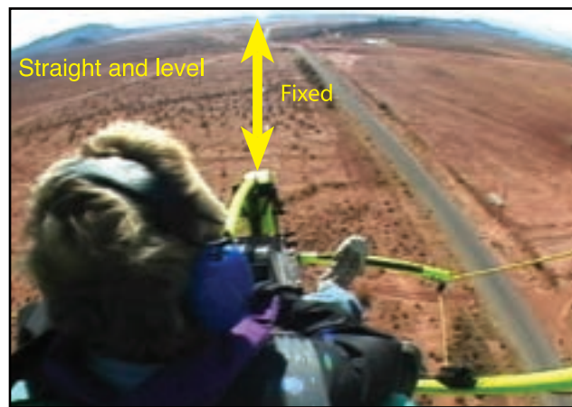
Figure 6-3. PPC attitude is based on relative positions of the aircraft on the natural horizon.
