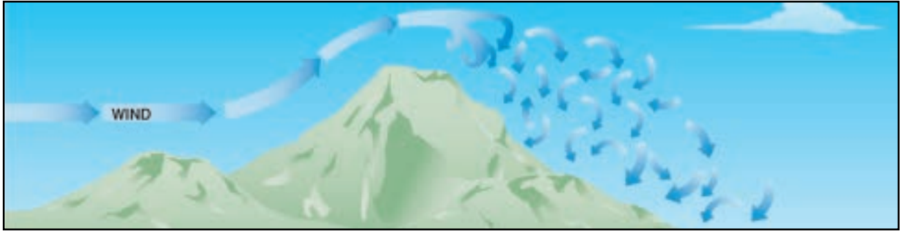
Figure 5-3 continued. Turbulence encountered over manmade items and in nature.
