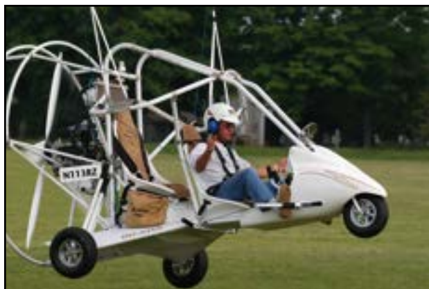
Figure 12-7. Engine-out, beginning full-flare about one second above the ground.
