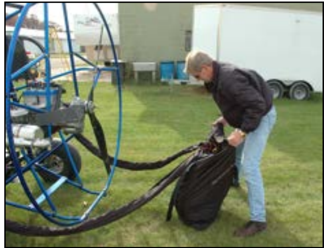
Figure 5-24. The line sleeve on the side of the cart where the bag will be stored can be placed on top of the folded wing, inside the bag; the other line sleeve will be used to store the bag on the cart.
