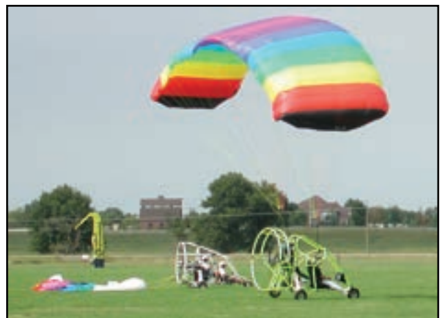
Figure 7-3. Pressurizing, or kiting, the wing.
