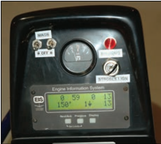
Figure 3-7. Typical engine information system.
