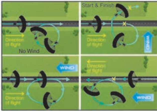
Figure 9-3. Effect of wind during turns.
