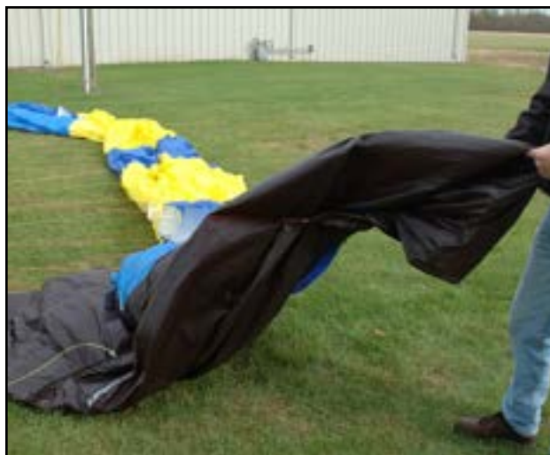
Figure 5-21. A simulated line-over.
