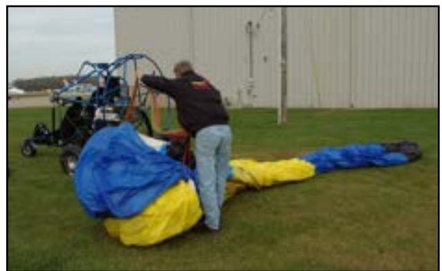
Figure 5-20. Pilot throwing the wing edge through to undo a line twist.
