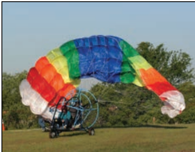
Figure 7-4. The powered parachute should be headed into the wind during takeoff.
