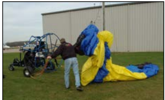
Figure 5-19. Undoing a line twist—beginning of the process.
