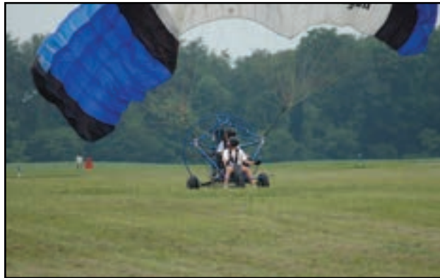
Figure 11-7. Collapsing the parachute.
