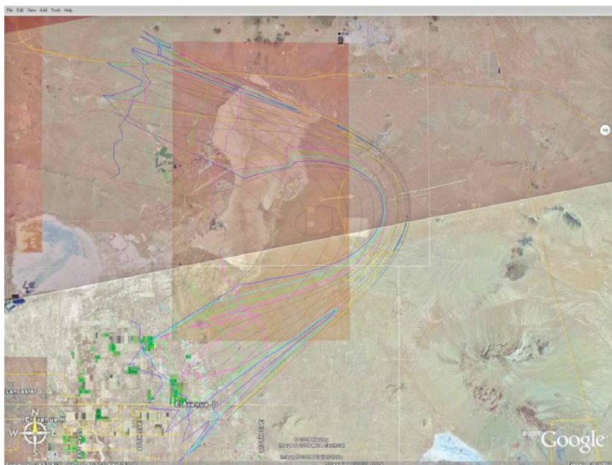
Figure 11. Low-boom dive sonic boom footprint superimposed on GoogleEarthPro TM map.
