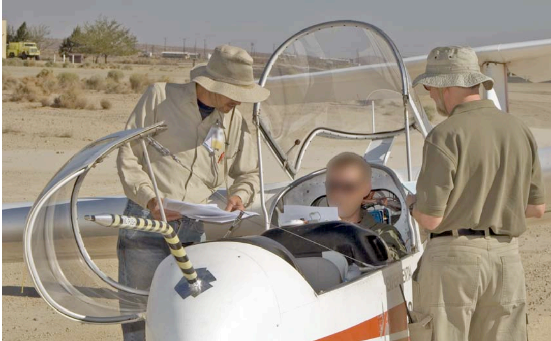
Figure 6. The sailplane's noseboom-mounted microphone and bullet-nosed windscreen.
