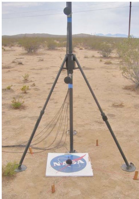
Figure 3. The 10 m tall tower with microphones at 1.2 m and 0 m; 2 ft by 2 ft by 0.75 inch groundboards were used under the ground-level microphones.
