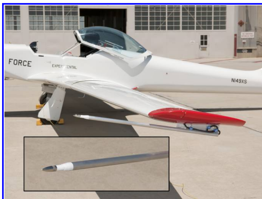
Figure 8. The wingtip-mounted microphone on the TG-14 motorized glider, with inset closeup of microphone.
