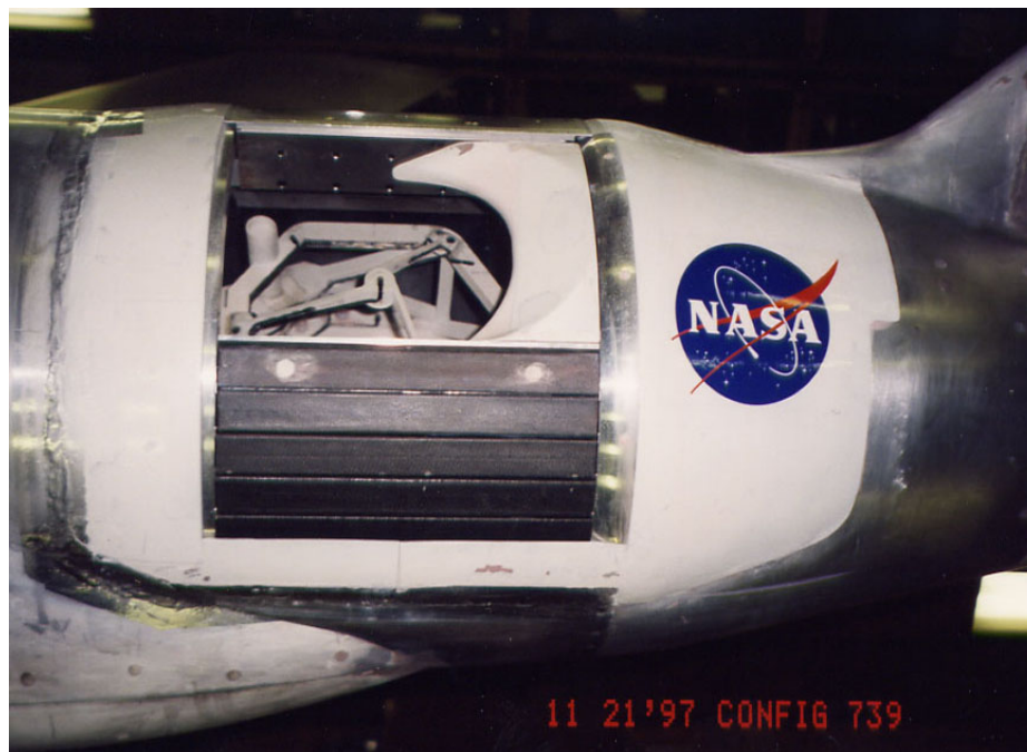
Figure 5. Partial external door configuration wind-tunnel model.
