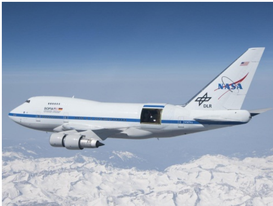
Figure 4. The SOFIA airplane flying in an open-door configuration.
