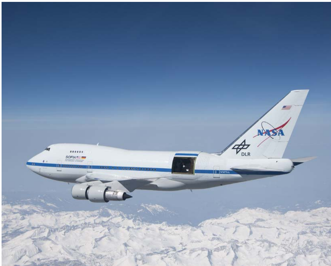
Figure 3. SOFIA cavity door system.
