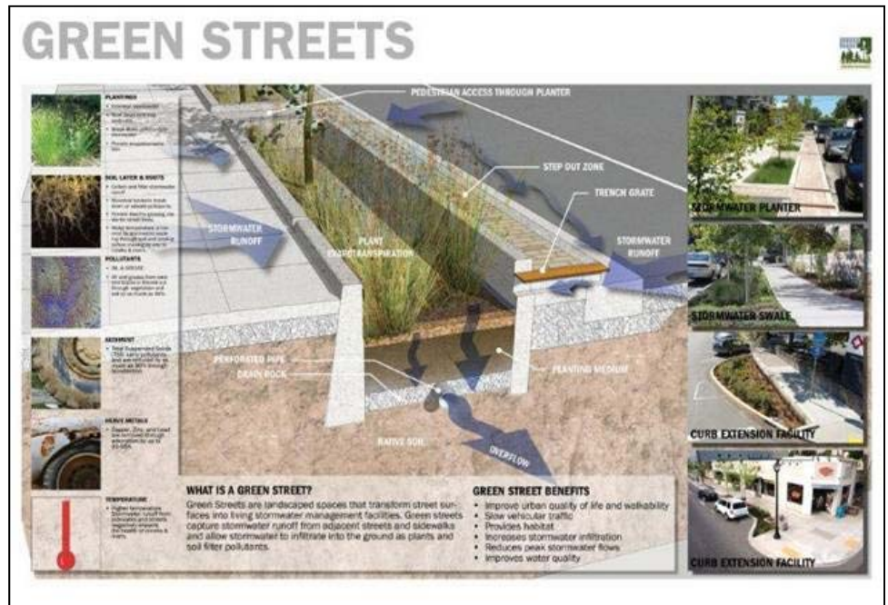
Illustration of a number of different versions of green street treatments. The cutaway shows how water flows into a rain garden and then flows through the rain garden
