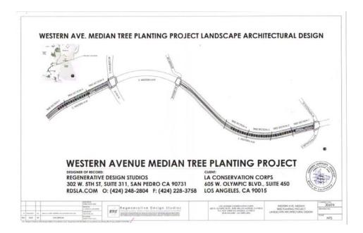
The project was funded by Council District 15 at approximately \$150,000 to remove 10 ft. x 10 ft. sections of asphalt paving within these raised median areas. Two (2) species of small stature trees were selected in coordination with CD 15, and planted in an alternating pattern approximately 30 ft. apart. The planting area was then covered with 3 inches of shredded cedar mulch to conserve moisture within the soil.
