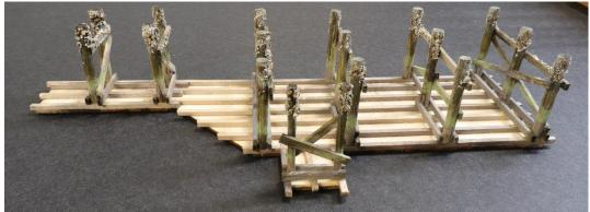
14. Now for most of this step you will use 1/32" x 3/32" stripwood (PURPLE tip) to add a variety of cross bracing between the different leg assemblies. But it can be different sized stripwood to fit the situation. Now is a good time to use up some of your scrap cutoffs. It all adds variety, just as in the prototype. They would use whatever was available if the dock were moving around and they needed to sure it up.
