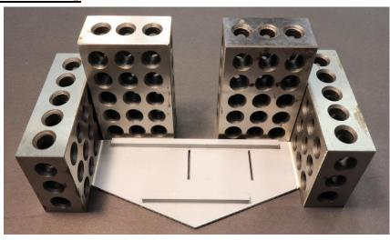
9. An important part in ensuring that the walls turn out square is to use two 1-2-3 blocks while gluing up the end gable wall (part #4). Be sure before gluing on the side wall, that your clapboard is facing the right way (see photo). You do not want to have the clapboard facing upside down. Having the 1-2-3 blocks against the long wall, glue the short gable walls to the 1/16" corner trim. This will create a 90-degree angle, ensuring your building will be square.
