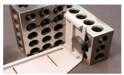
10. After the 3 walls are dry, the remaining front wall (part #3) can be glued to the opposite ends of the short walls. Again, use the square and blocks to keep everything aligned.
