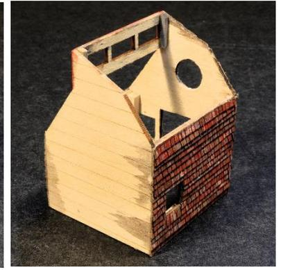
97. Paint, glaze and install the windows and door. It will take a little tweaking of the shingles around the openings to get them to fit properly.
