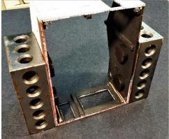
7. The garage assembly is next. This requires parts #5,6,7. Lay part #5 clapboard side down. Using 1-2-3 blocks and magnets, glue peaked walls #6&7 to the short sides of #5, being sure to align the bottom of the walls. The 2 slots on #5 are closer to the bottom. This allows the
