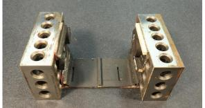
8. Now take parts #8, 9, 10 to build the small lean-to. This is a very similar step to the garage build. Lay part #8 scribed side down. Using the 1-2-3 blocks and magnets to glue on the sloped sides to the outside edges of part #8.
