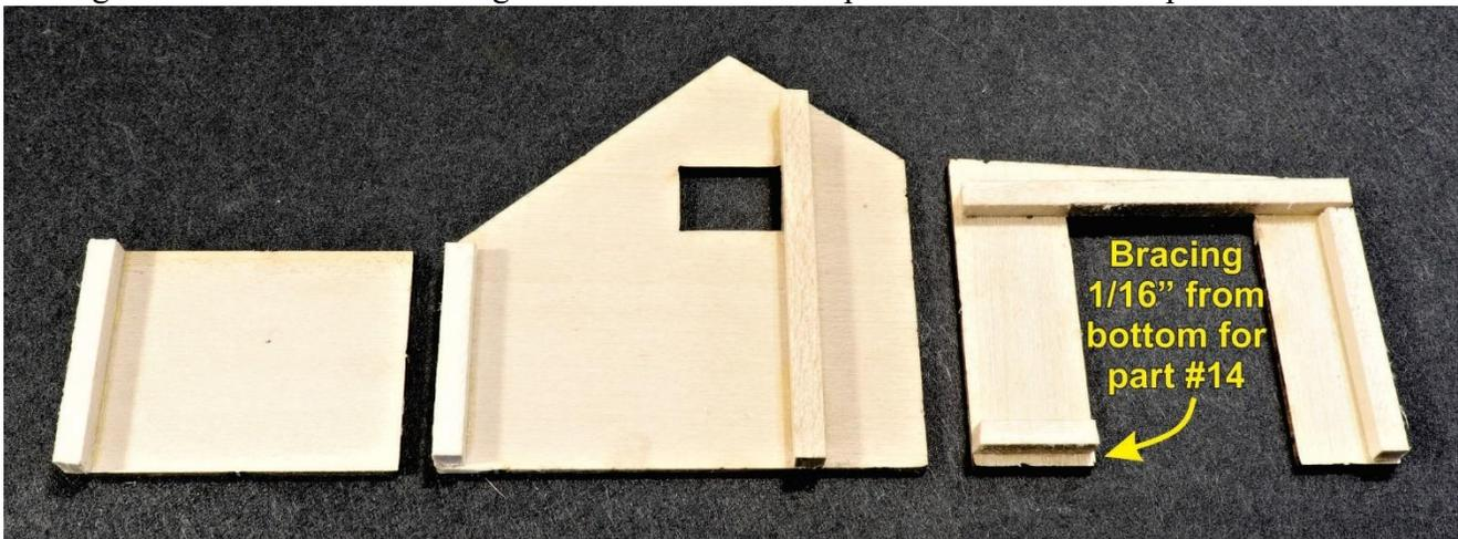
22. Add part #14 (x2) to the back of #12. These reinforce the 45-degree wall joint. One goes on the bottom underneath the bracing, and one goes on top of the top bracing. (see right)
