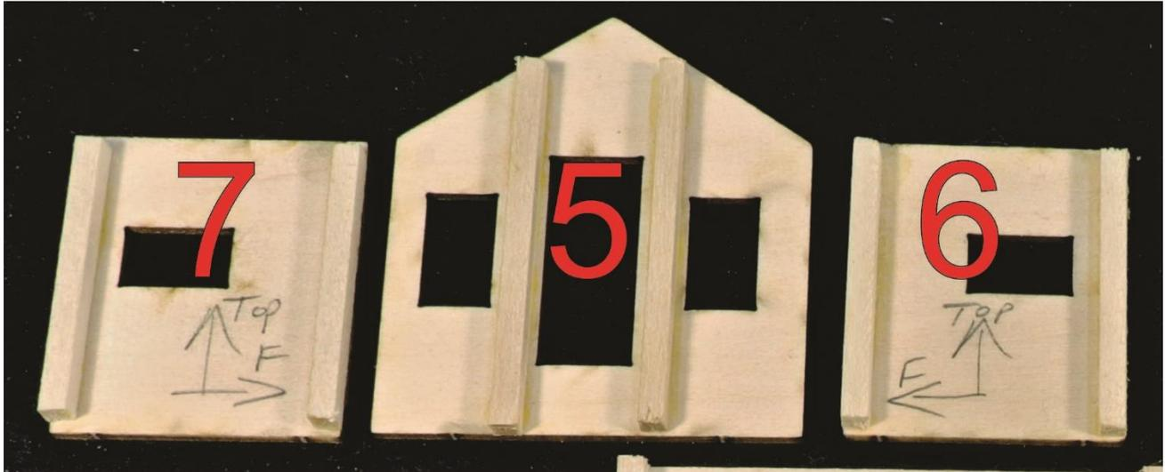
18. Add 1/16" x 1/16" corner trim to the sides of part #5. Once dry, use the 1-2-3 blocks to join #6,7 to the back side of #5. File the top edges of #6,7 to match the pitch of the gable on #5. This makes fitting the roof easier and more precise. (see right)
