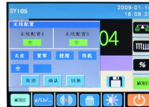
4) Wireless Sensor Mode. Without touching and just waving hands above the screen, tare, zero, calibration and power on/off can be finished.
