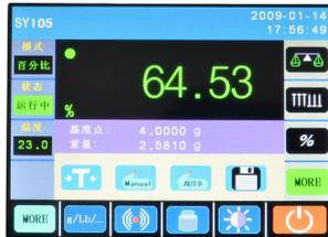
3) Percent Weighing Mode. Tare and storage function available, Manually or automatically defined for the reference point can be achieved.
