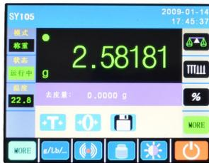
1) Weighing Mode. In this work mode, results can be displayed and stored, also Tare, Zero function available.
