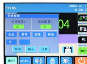
4) Wireless Sensor Mode. Without touching and just waving hands above the screen, tare, zero, calibration and power on/off can be finished.
