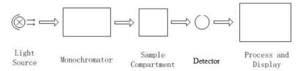
Fig 2.4 Block diagram for the Spectrophotometer
