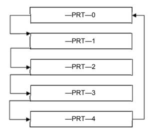
PRT-O is an output mode with indefinite time. Then press the button <PRT>, the weighing result will be output from the interface.
