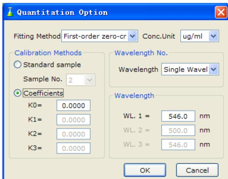
2. Put the sample into the light path, select the menu <operation> <Set Blank> or click the shortcut toolbar buttons [ Set Blank], instrument will be set to the operating wavelength, and set blank 0.000 Abs/100.0 %T. Coefficient formula is shown as follows.
