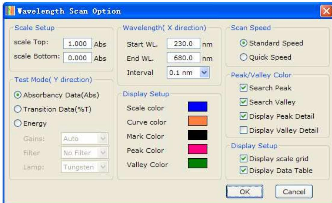
3. Select display mode (Select the energy scan mode, the proposal is set to a fixed Gain), scanning the wavelength range, coordinates the upper limit, lower limit coordinates and scanning interval.
