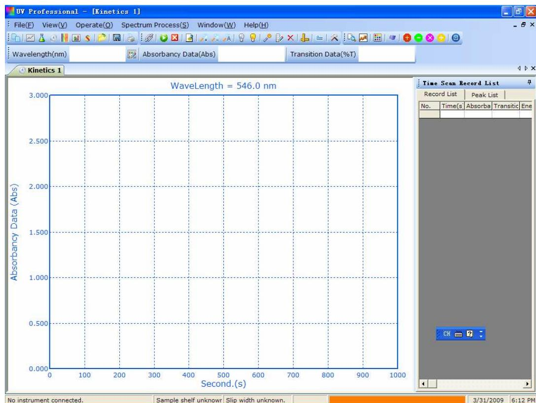
2. Click shortcut toolbar [
