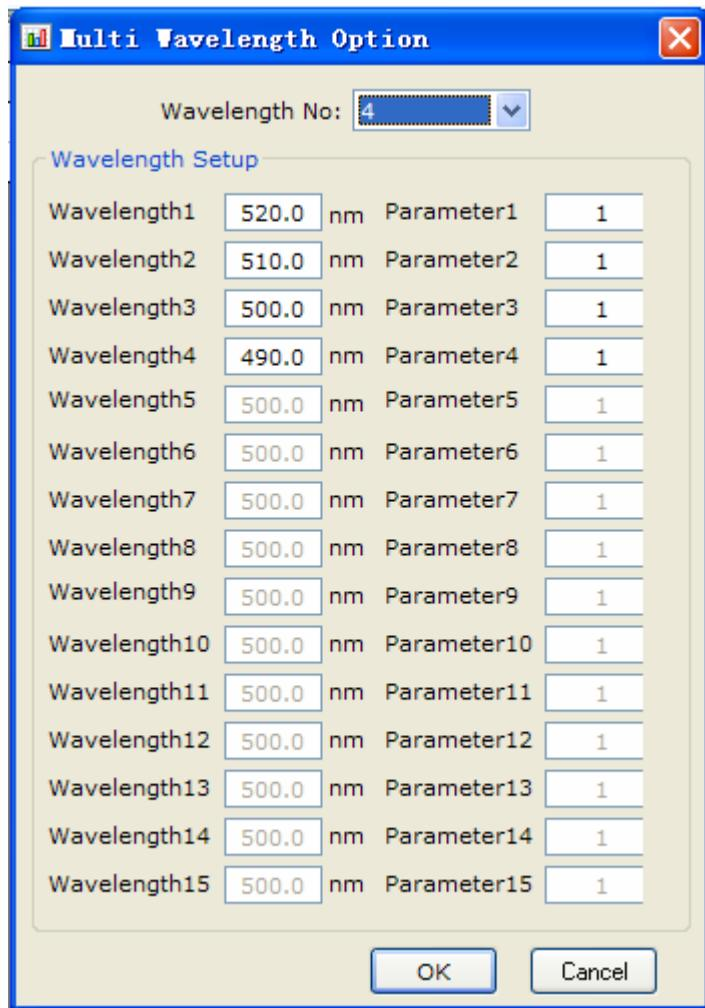
3. Input wavelength number, and Input coefficient:
