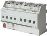
Rated contact current according to DIN EN 60669: 10 AX (140 µF fluorescent lamp load), 10 A (resistive load)
