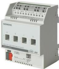
Rated contact current according to DIN EN 60669: 16 AX / 20 AX (200 µF fluorescent lamp load)
