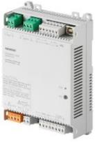
Compact room automation station, BACnet/MSTP, 230 V, flat housing, 1 DI, 2 UI, 1 relay, 1 AO, 4 triac
