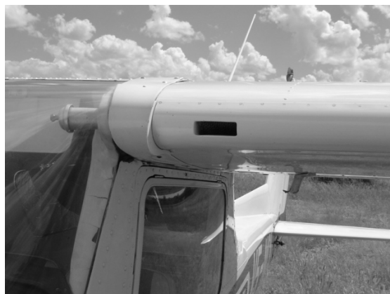
Check top and bottom wing surfaces for any damage or accumulations on wing. Ice or excessive dirt must be removed before flight.
