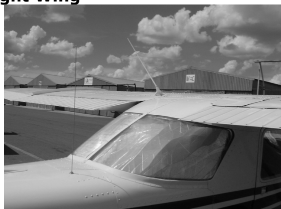
Check top, bottom, and side surfaces for any damage. Aerials undamaged and secure.
