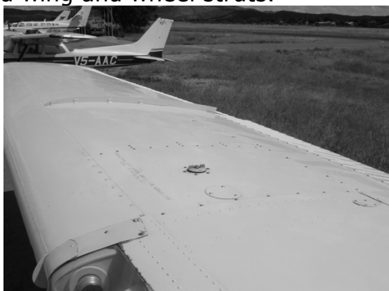
Check that fuel cap is secure. (For the type shown the grip should be inline with the longitudinal axis of the aircraft.)
