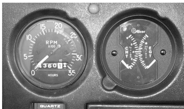
Illustration 5e Tachometer and Modified Post-manufacture CHT/EGT Gauge
