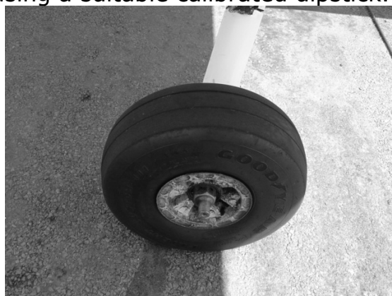
Check tyre for wear, cuts, bruises, and slippage. Recommended tyre pressure should be maintained. Remember, that any drop in temperature of air inside a tyre causes a corresponding drop in air pressure.
