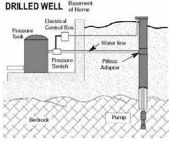
with at least 5 feet extending into the bedrock. The casing should also extend a foot or two above the ground's surface. A sealant, such as cement grout or bentonite clay, should be poured along the outside of the casing to the top of the well. The well should be capped to prevent surface water from entering the well.
