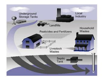
Septic tanks are designed to have a leach field around them, which is an area where wastewater flows out of the tank. This wastewater can also move into the ground water.
