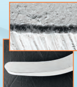
Cutting edge of the LM Sharp Diamond™ curette and the magnification of the edge after the test.
